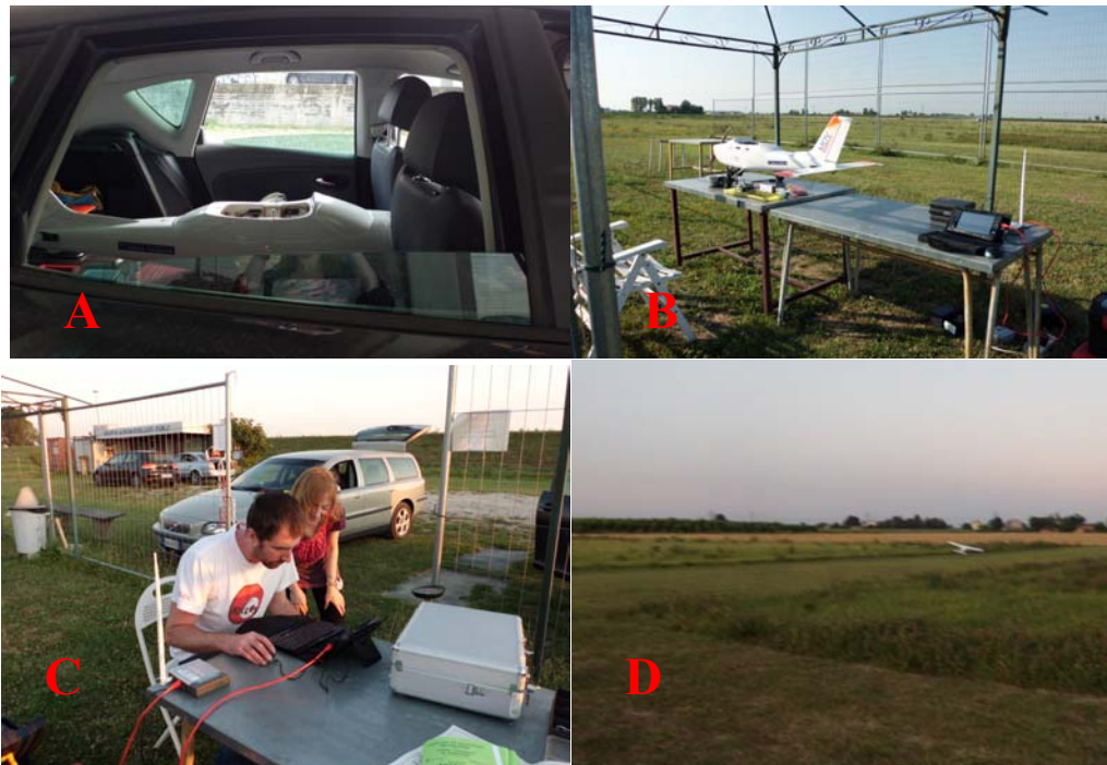
Figure 7 Flight test at Gruppo Aeromodelлисти di Forlì strip on June 30 2011: a) Cardinal lodged on the car; b) Final assembly phase; c) Telemetry and acquisition software testing; d) Cardinal Take Off.
