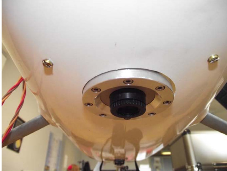
Figure 6. External view of the Thermal Eye 3600 AS fixed on the Cardinal fuselage.
