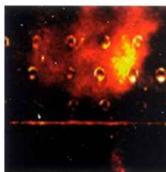
Corrosion of 737 lap joint
