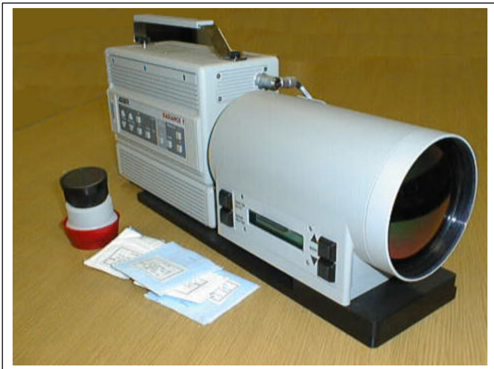
Figure 5: 3-5 micron band, 12-bit, infrared video camera, "Radiance 1" from Amber Engineering, with SiGe 75-250 mm f2.3 telephoto lens and internal filter wheel, all controlled by an RS-232 port. Standard 50 mm f2.3 lens is next to some of the filters.
