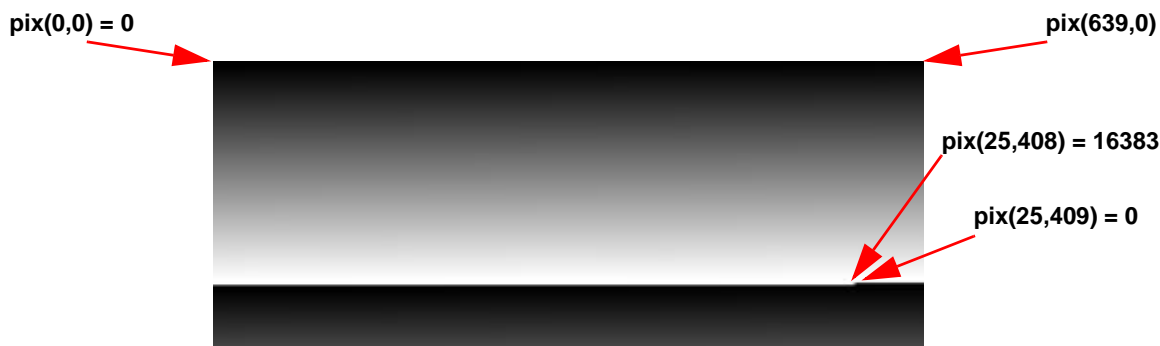
Figure 3-5: Ramp test pattern example for Top Portion of Photon 640 Slow Video Ramp Image (Digital values shown apply to the optional 14-bit digital data stream.)
