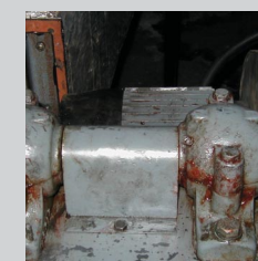
Mechanical: Overheating bearing at pulley end
