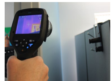
Missing insulation with E60 thermal imager.
