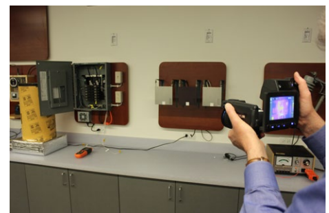
310:1 SSR = 77.5" from target Figure 4. Note: Breaker panel above is touch safe.
