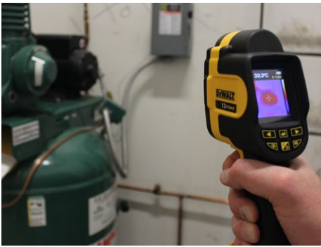
With a 6:1 spot size ratio, this device is better suited for large targets. Figure 7.
