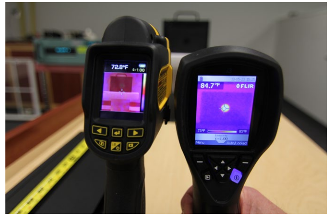
From 30" away, we looked at both from a detection only standpoint. We could still see the thermal image of the 1" target clearly with the i3 (right) but could only faintly detect it with the Imaging Thermometer, which had the IR blended with its visible picture (left).
