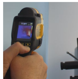
Missing insulation with imaging thermometer.
