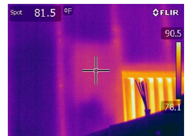
From 30" away, we looked at both from a detection only standpoint. We could still see the thermal image of the 1" target clearly with the i3 (right) but could only faintly detect it with the Imaging Thermometer, which had the IR blended with its visible picture (left).
