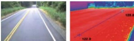
**Cooling asphalt mat** - With only a 3 Fahrenheit degree differential, the longitudinal section shown in the thermograph indicates that this cooling asphalt mat exhibits exceptional thermal uniformity. The mean density of this asphalt mat is 2,205 kilograms per cubic meter, with a maximum of 2,247 kg/m<sup>3</sup> and a minimum of 2,179 kg/m<sup>3</sup>. The visual photo of the road taken a year later shows no evidence of wear or degradation.
