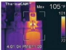
**Electrical** - Infrared testing is used as a means to detect potential circuit overload or areas of unusually high electrical resistance, allowing electricians to replace the circuit before failure, eliminating costly downtime or further damage to the electrical system.
