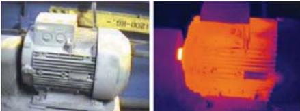
**Preventative Maintenance** - Plant maintenance technicians use infrared testing as a form of preventive maintenance by monitoring a variety of machine parts. By evaluating a machine's temperature signatures when in normal operating conditions, one can perform periodic infrared inspections to detect overheating joints, bearings, etc. in order to avoid costly downtime. This kind of preventative or predictive maintenance is critical to increasing & maintaining plant efficiencies.
