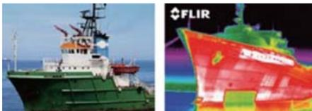
**Boat** - An IR camera can detect alterations made to vessel structure. Image shows a plate welded to the hull.
