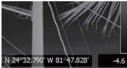
Graphs 4.11a Camera automatically adds position data to each IR-image
