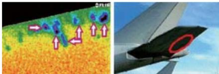
*Graph 3.0 Thermogram showing water ingress (dark areas) on illustrated section of aircraft. An entire aircraft can be surveyed in 20 minutes with no downtime. Images are recorded digitally for later analysis at an image processing workstation.*
