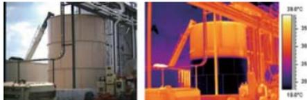
**Liquid storage tank** - An IR camera can show when there are multiple levels in a tank, allowing workers to determine whether or not the product is contaminated or the tank itself needs to be serviced. This allows them to optimize the product. And when weather conditions are optimal, leaks from PRV's, steam, hot gases and propane can be illuminated.
