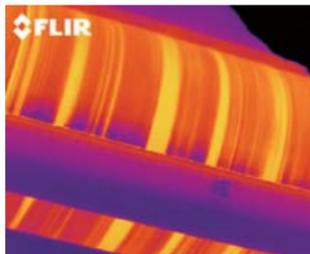
**Paper Web Process** - Thermal image of a paper web process. Moisture shows up clearly in the image.
