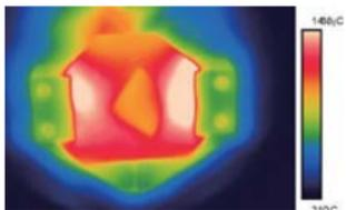
**PC Board** - PC board with overheating component.
