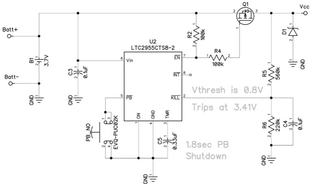
The power supply circuit allows the user to turn the power of the tool on and off. That is especially important for conserving power in a small battery powered tool. Here, again, we use an IC to do the heavy lifting, in this case [Analog Devices LTC2955](#) which is a Pushbutton On/Off controller.
