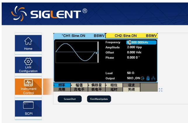
Supports control of the instrument through a Web browser, allowing testing tasks to be accomplished remotely.
