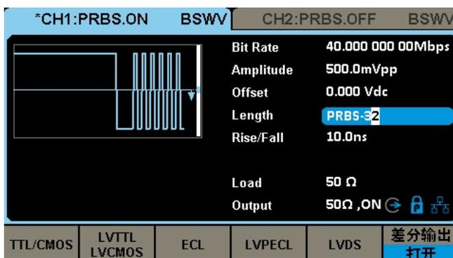
Quickly select preset level logic such as TTL, LVCMOS, LVPECL
