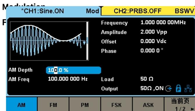
Rich modulation functions, support commonly used AM/DSB-AM/ FM/ PM/ ASK/ FSK/ PSK/ PWM modulation mode
