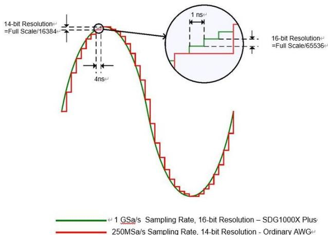
16-bit, 1 GSa/s sampling system with high resolution in both time and amplitude for maximum waveform detail and distortion avoidance
