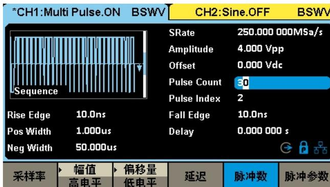
Supports a maximum of 30 pulses, each pulse can be set independently of the pulse edge and positive and negative pulse widths
