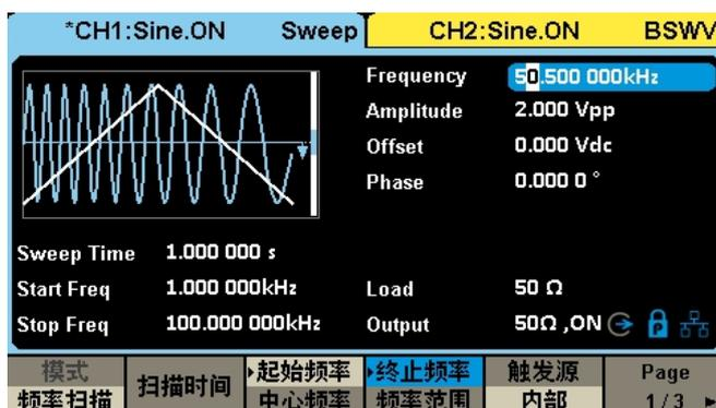
Supports two Sweep modes of frequency and amplitude, easily realizing frequency sweep and amplitude sweep.
