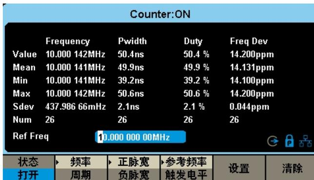
Highly accurate frequency meter with a frequency range of 0.1Hz to 200MHz.
