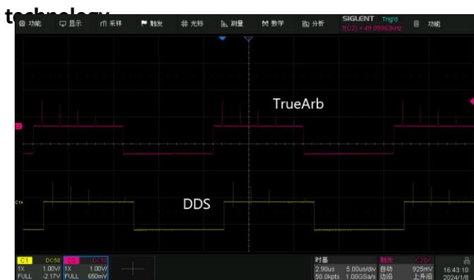
TrueArb not only has all the advantages of traditional DDS technology when outputting arbitrary waveforms, but also overcomes its serious shortcomings that can increase jitter and distortion because TrueArb technology outputs every waveform data point of an arbitrary waveform in memory point by point, without missing any details, and accurately generates arbitrary waveforms with low jitter.
