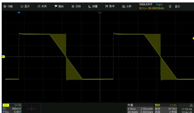
Rising and falling edges can be set separately; adjustable in steps as small as 100ps; minimum value of 10ns can be obtained at any frequency; maximum value up to 22.4s
