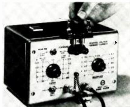
Forward current and reverse voltage on the tester is continuously variable through five ranges. Push-button control allows rapid forward and reverse testing. Reverse leakage and forward current is controlled to prevent overloading by use of limiting circuitry.
