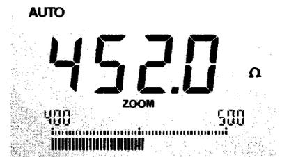
In this mode, the 0.4% resolution is virtually identical to a normal analogue multimeter, but with much higher accuracy and repeatability.
