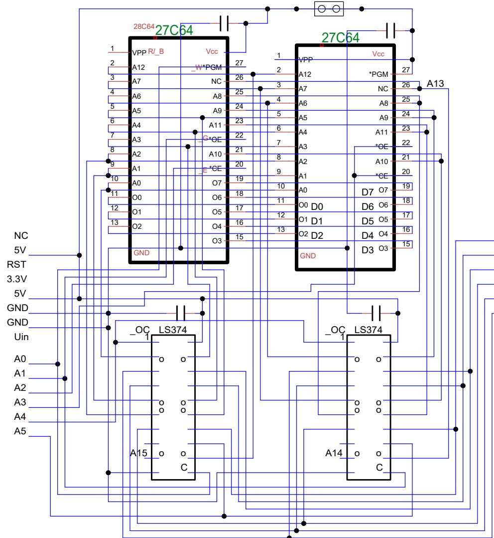
Copy 27C64 to 28C64, controlled by Arduino UNO
