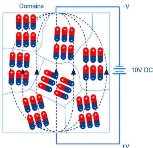
Figure 4 – BaTiO<sub>3</sub> under the influence of an electric field
