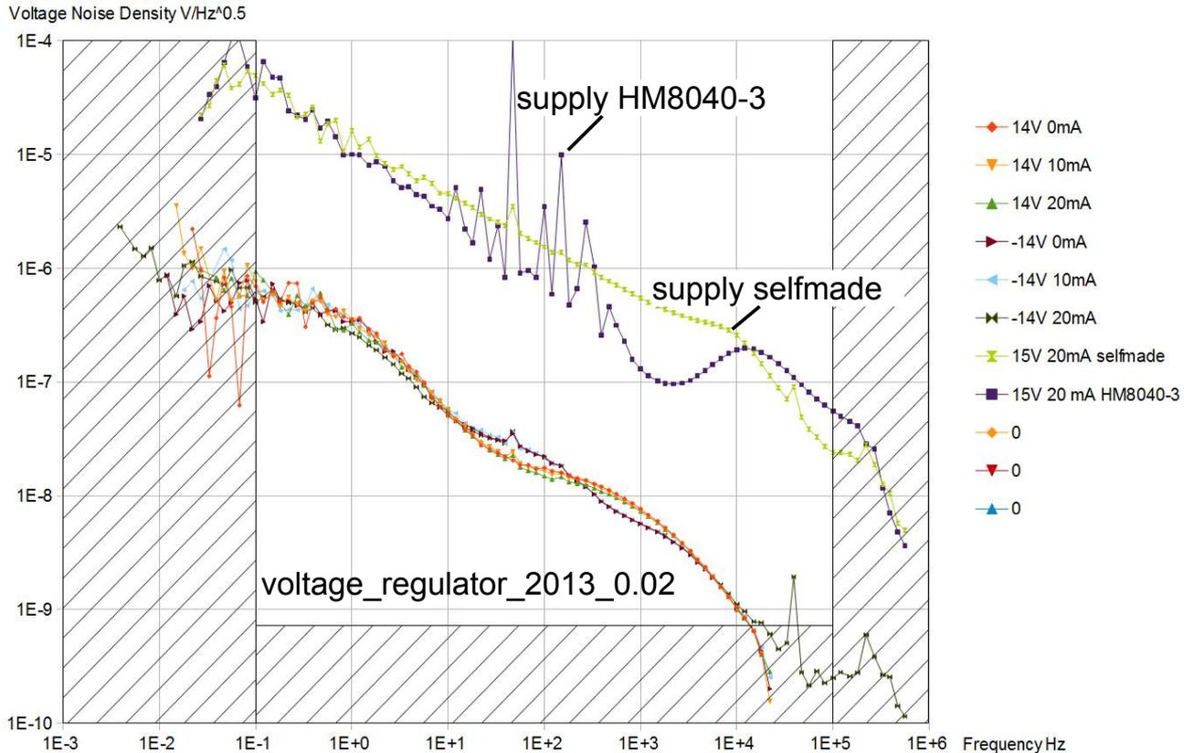
Figure 1 Voltage Noise Density of one prototype and two other supplies
