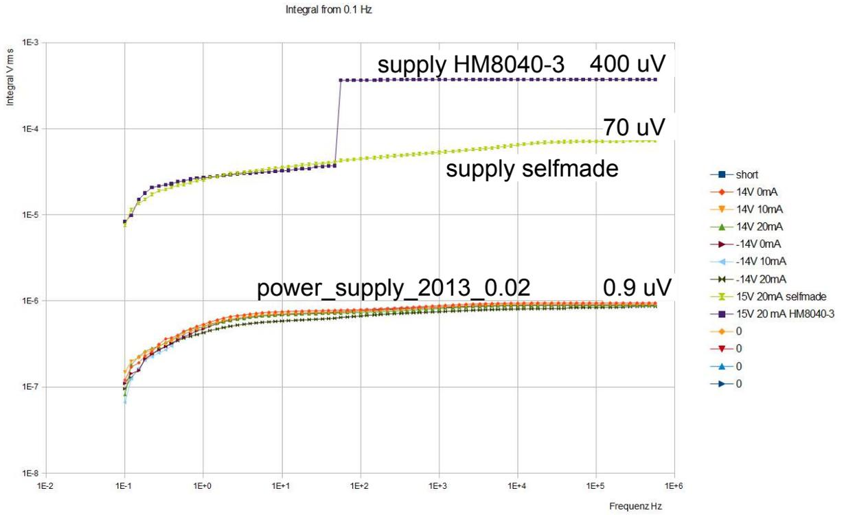
Figure 2 Voltage Noise, integrated from 0.1 Hz
