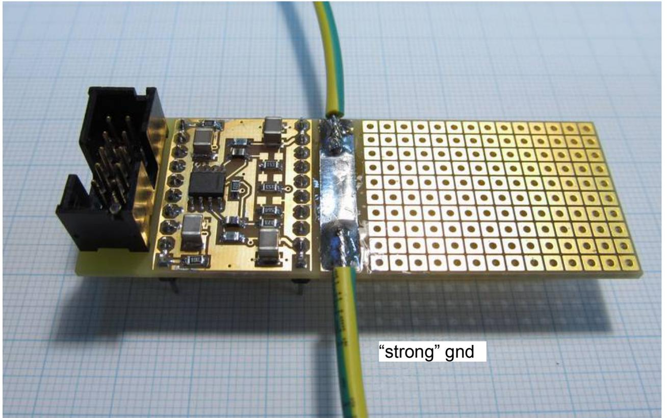
Figure 8 Example: gnd over wires.
