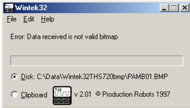
Error: After trying to receive data -> Port settings on PC were NOT correct
