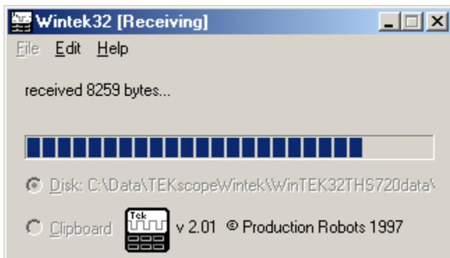
receiving DATA after pressing **HARD COPY on the TekScope**
