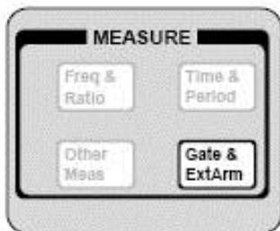
The SS7402 has two arming modes: Internal and External. Press **【Gate&ExtArm】** key until 1.000000 is displayed and the indicator light. Use **【↑】** and **【↓】** to increase and decrease values of current digit, use **【←】** and **【→】** to select digit needed to be adjust and specified range is 0.000001s to 1000s. After selecting, press **【ENTER】** to
