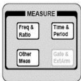
All measurement functions are realized by these three keys. Use **【Freq&Ratio】** to measure the Frequency and Frequency Ratio of CH1, CH2 and CH3. Use **【Time&Period】** key to measure Period, pulse width (Positive or Negative) and time interval. And use **【Other Meas】** key to measure count, duty cycle, phase difference and voltage.
