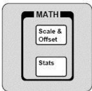
Math and Limits are not available for Count and self-check measurements. As shown in left diagram, the keys of **【Scale&Offset】** and **【Stats】** are included in **MATH** function area. The **MATH** function is disabled in the initial state and the indicator of the two keys are OFF.
