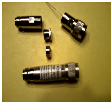
'N' connectors before (top) and after final assembly (bottom) with a label applied.
