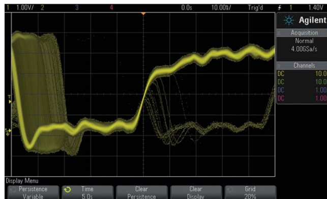
Figure 3: The Agilent MSO/DSO3000 X-Series oscilloscope reliably captures the infrequently occurring metastable state while updating at 1,000,000 waveforms per second.
