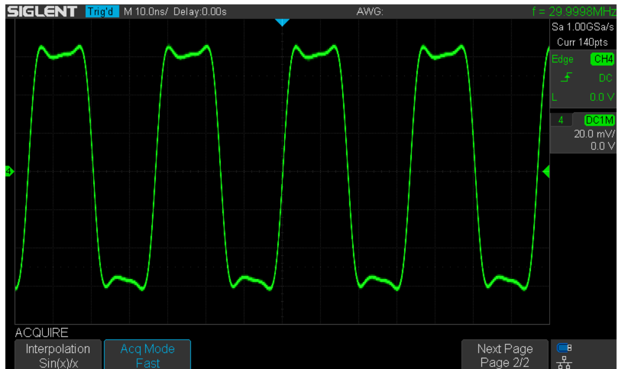
SDS1104X-E_Square_30MHz_10ns_fast_vectors
