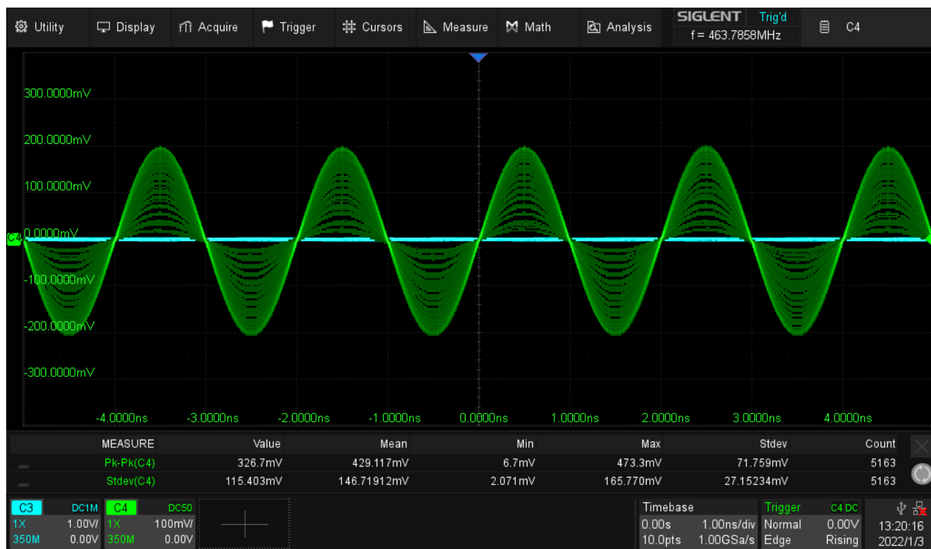
Figure 20. SDS2504X Plus_Sine_500MHz_BW350MHz_1GSa_SinX
