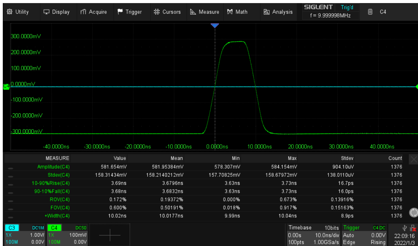
Figure 27. SDS2504X Plus_PR_B100M_1GSa_10MHz_W10ns_T1ns_10bit
