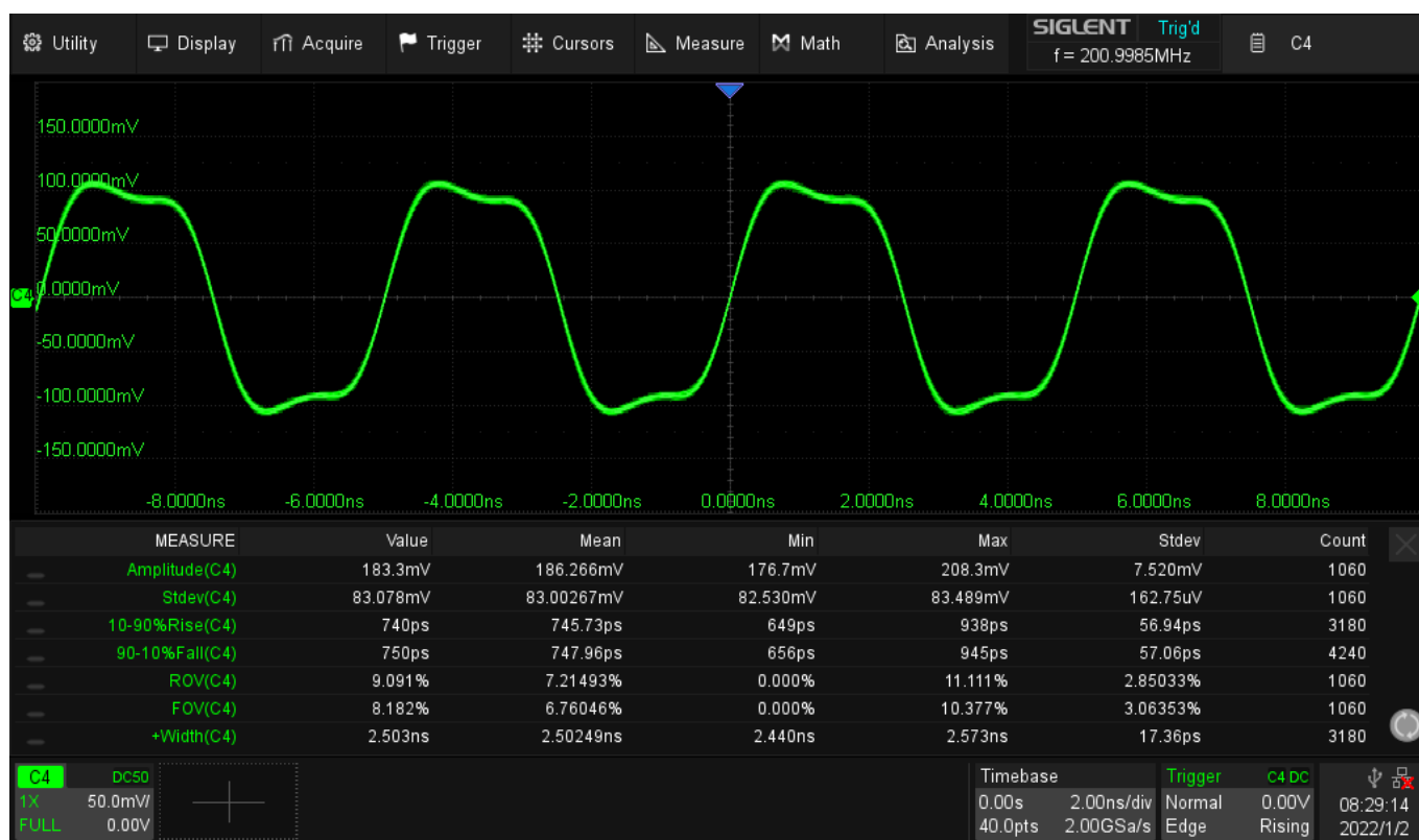
Figure 40. SDS2504X Plus_PR_B500M_2GSa_200MHz_Duty50_T200ps_V
