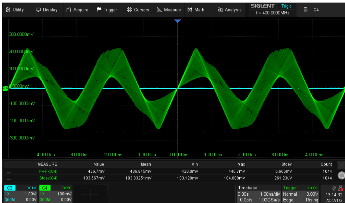
Figure 15. SDS2504X Plus_Sine_400MHz_BW350MHz_1GSa_X
