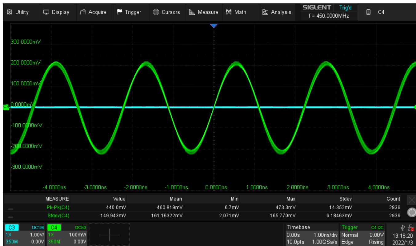
Figure 18. SDS2504X Plus_Sine_450MHz_BW350MHz_1GSa_SinX
