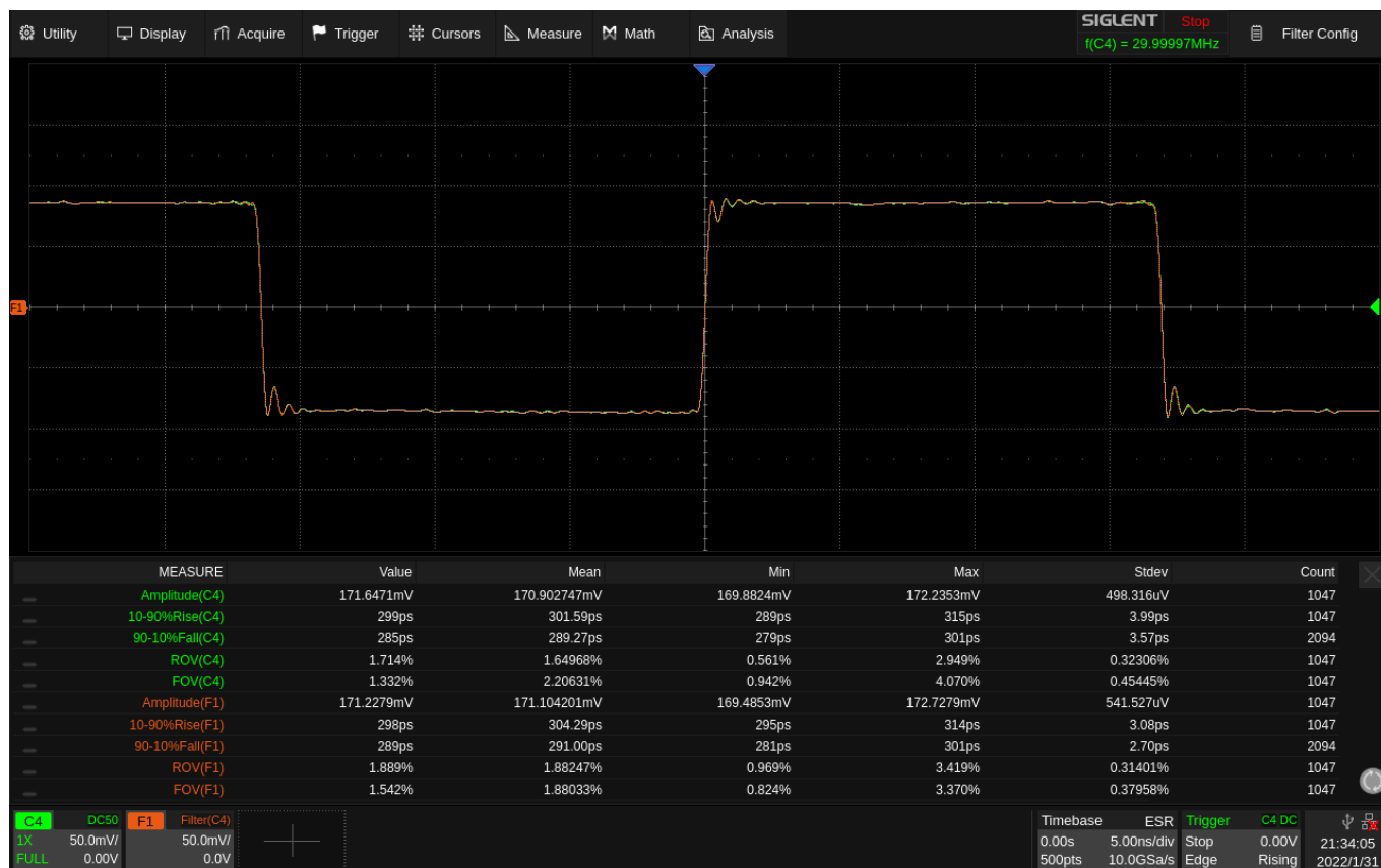
Figure 5. SDS6204_PR_30MHz_170mV_200ps_BW2.2GHz
