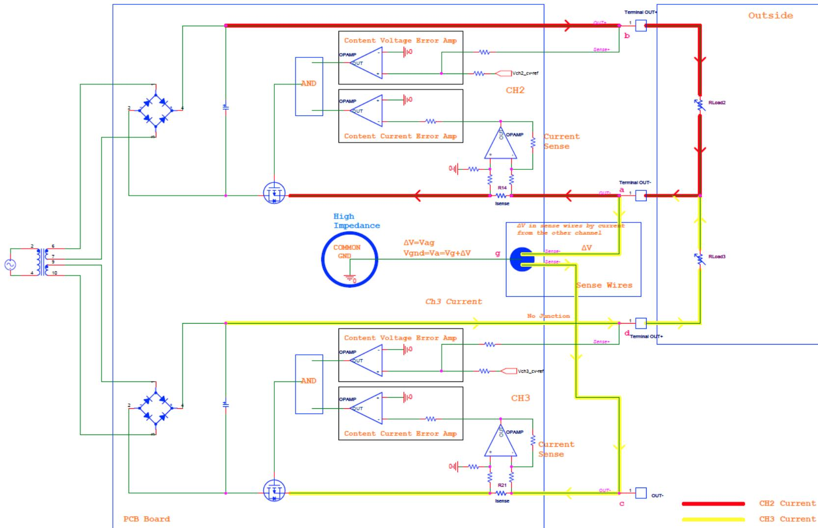
Note that in the cross-connection method (the positive terminal of RLoad3 is connected to the Terminal OUT+ of CH3 and the negative terminal is connected to the Terminal OUT- of CH2).
