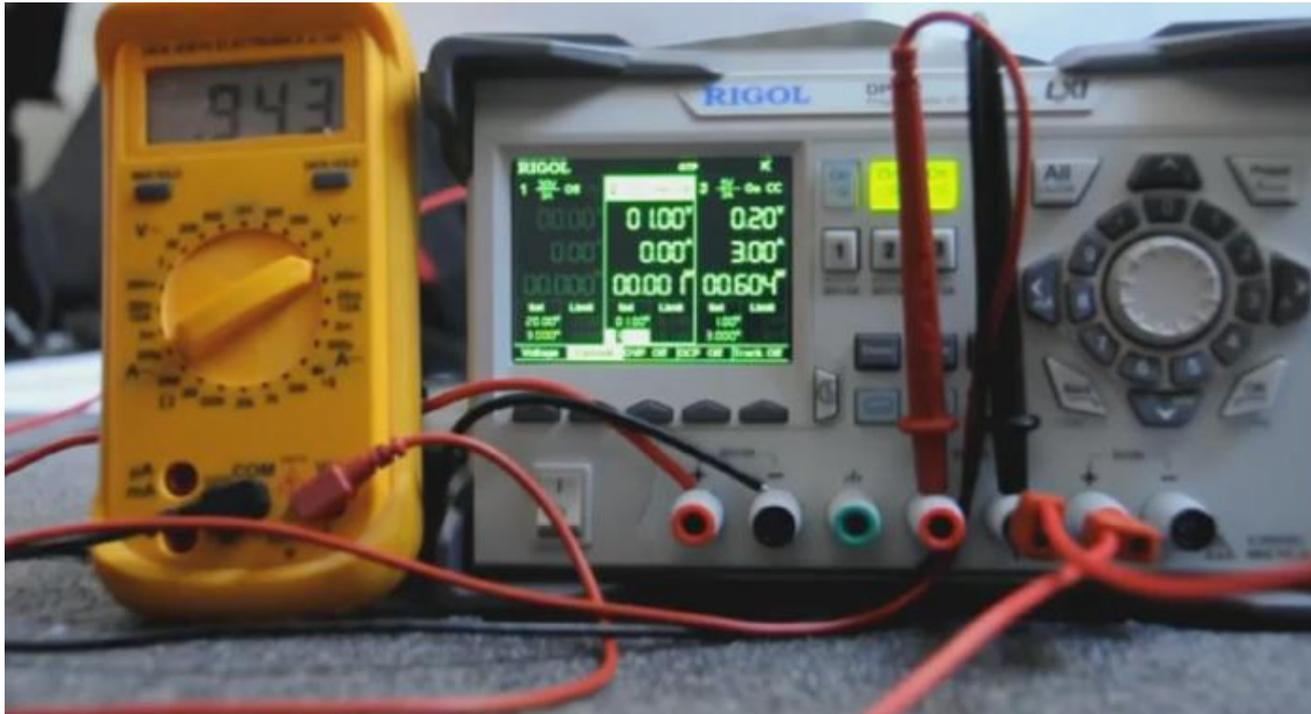
**Even** if you ground the 2 lows together externally, the voltage drop is out of spec for channel 2.
