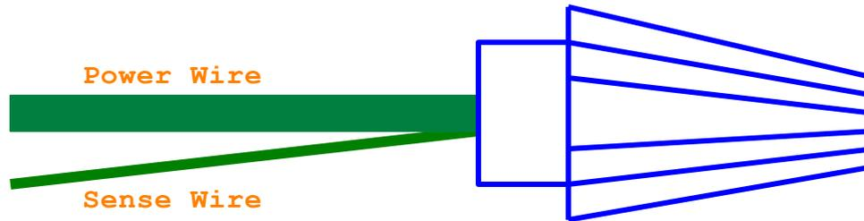
The Power Wire delivers the current, and the Sense Wire is fed back to the voltage from the Terminal.
