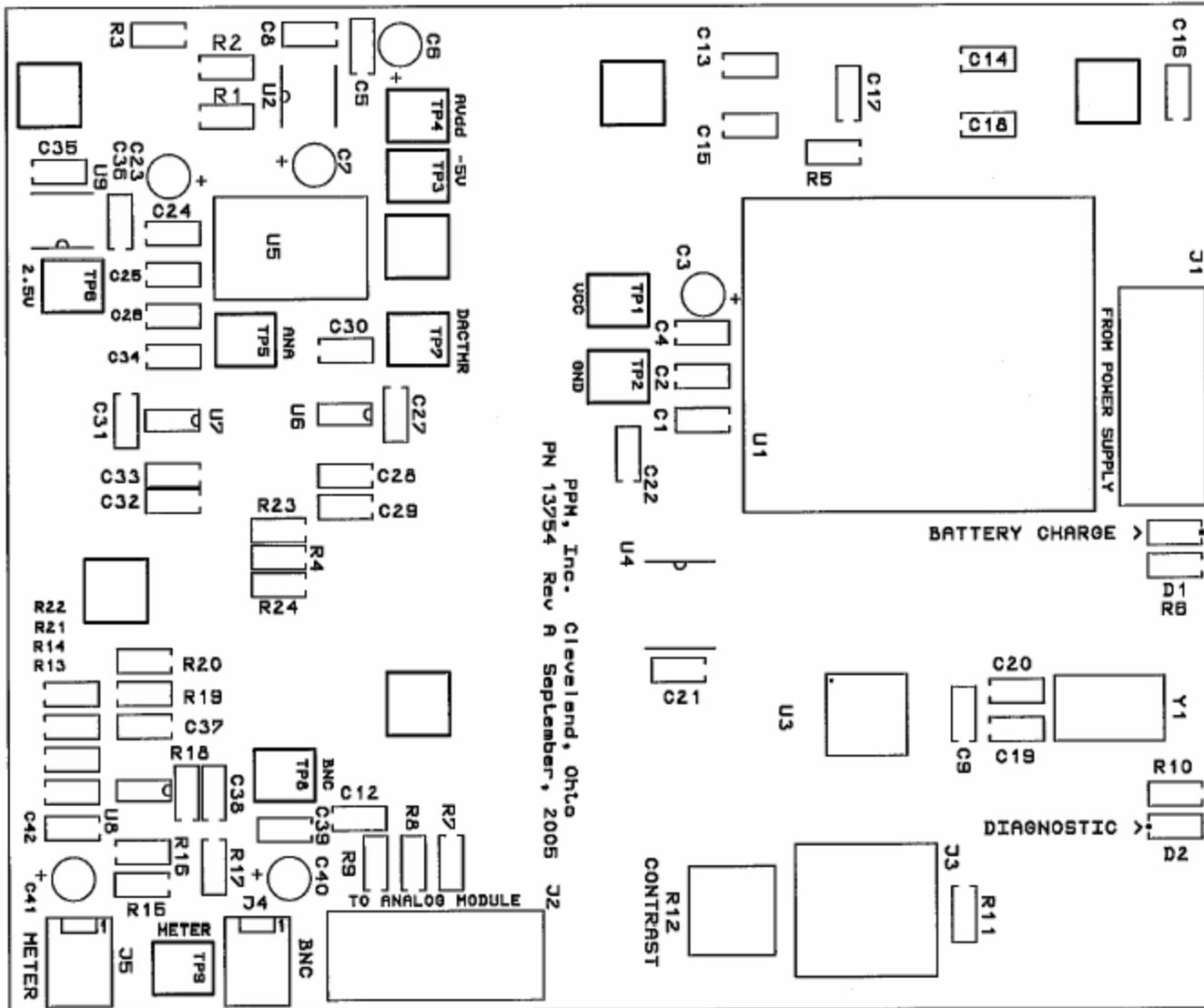
16.12. Circuit Board Parts Layout – Power Supply Subsystem
