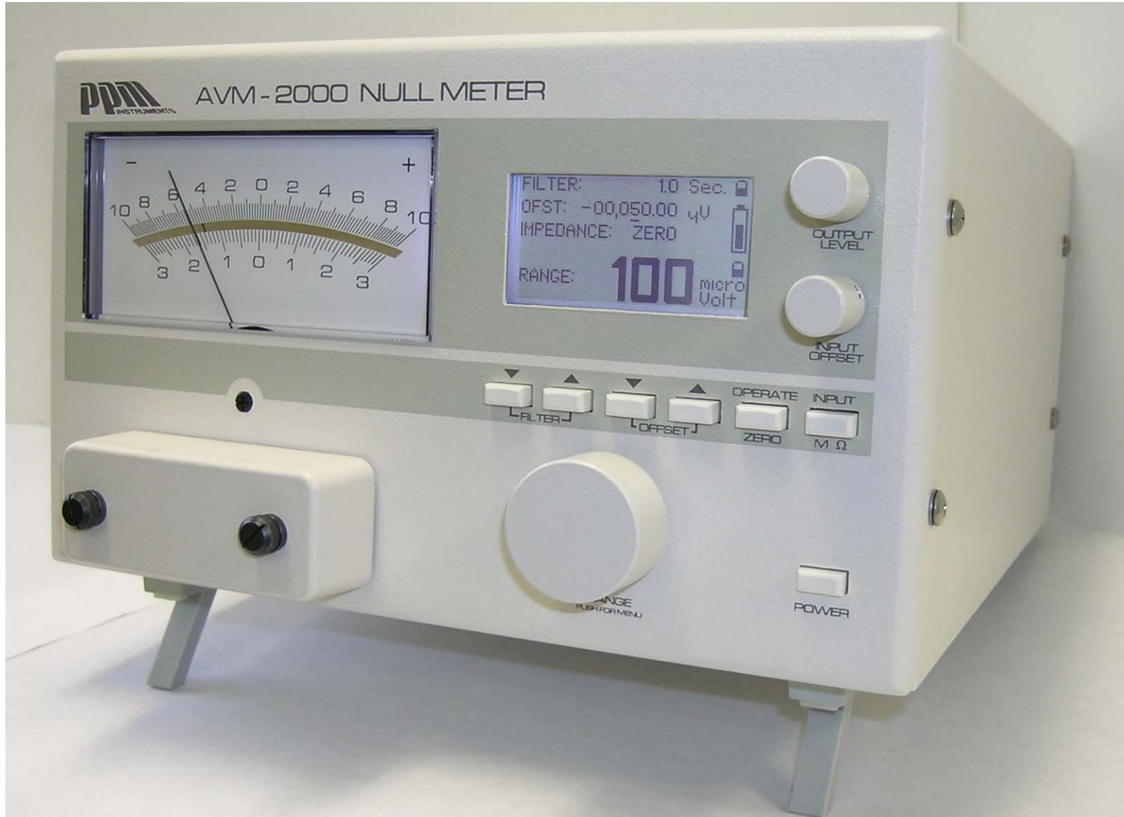
17.2. AVM-2000 Front View with Accessory Terminal Cover Box Installed
