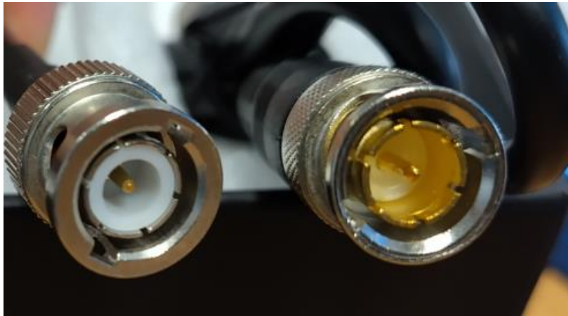
Figure 3 Left – 50 \Omega BNC, right – 75 \Omega cable supplied
