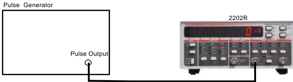
Figure 5-11, Delay Test Set-up.
