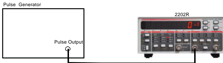
Figure 5-10, Auto Trigger A and B Test Set-up.
