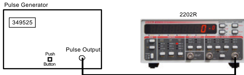
Figure 5-9, Totalize B Test Set-up.
