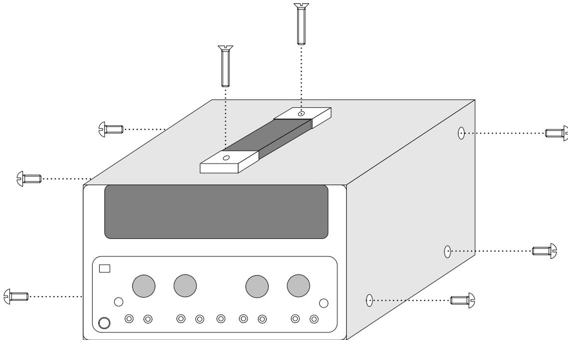
3. Hold the case, slide it behind, and pull it off upward.
