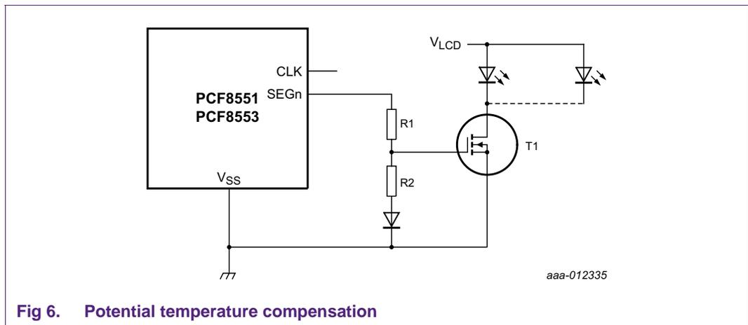
Fig 6. Potential temperature compensation
