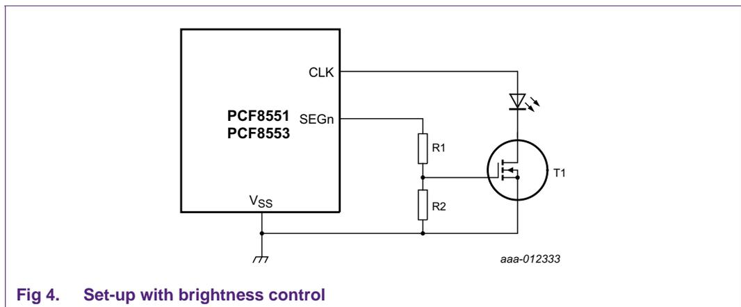
Fig 4. Set-up with brightness control
