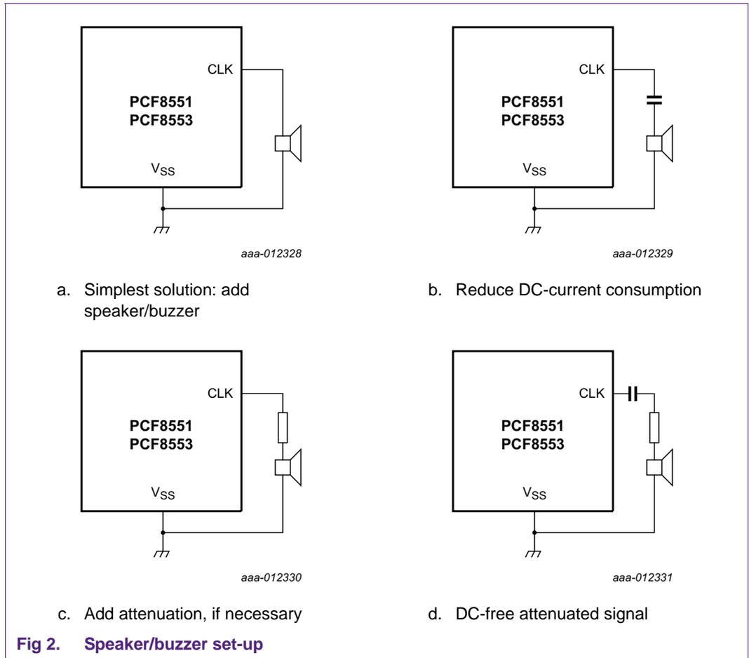
Experiments with an 8 Ω speaker showed reasonable performance. It is also possible to drive a capacitive buzzer.
