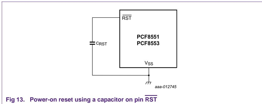
Fig 13. Power-on reset using a capacitor on pin  $\overline{\text{RST}}$
