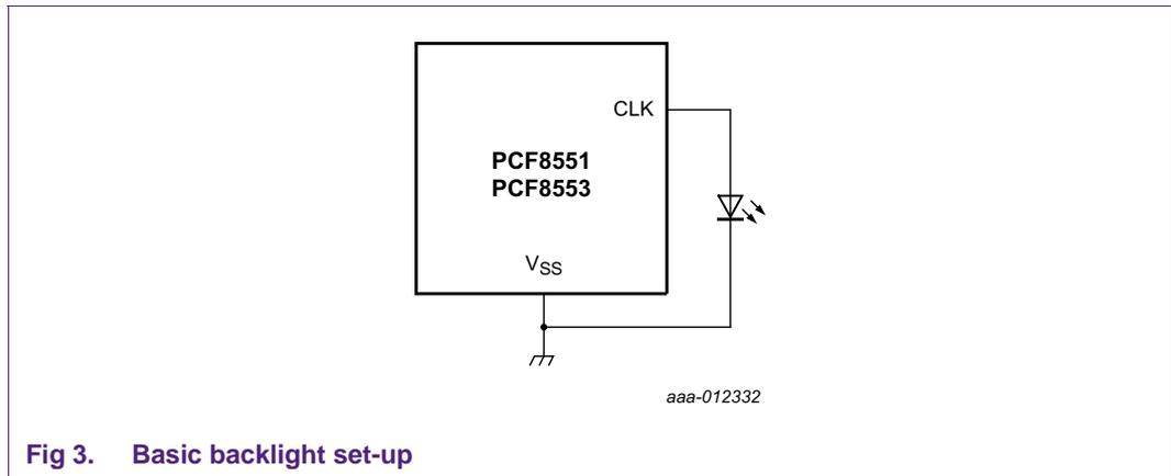
Fig 3. Basic backlight set-up
