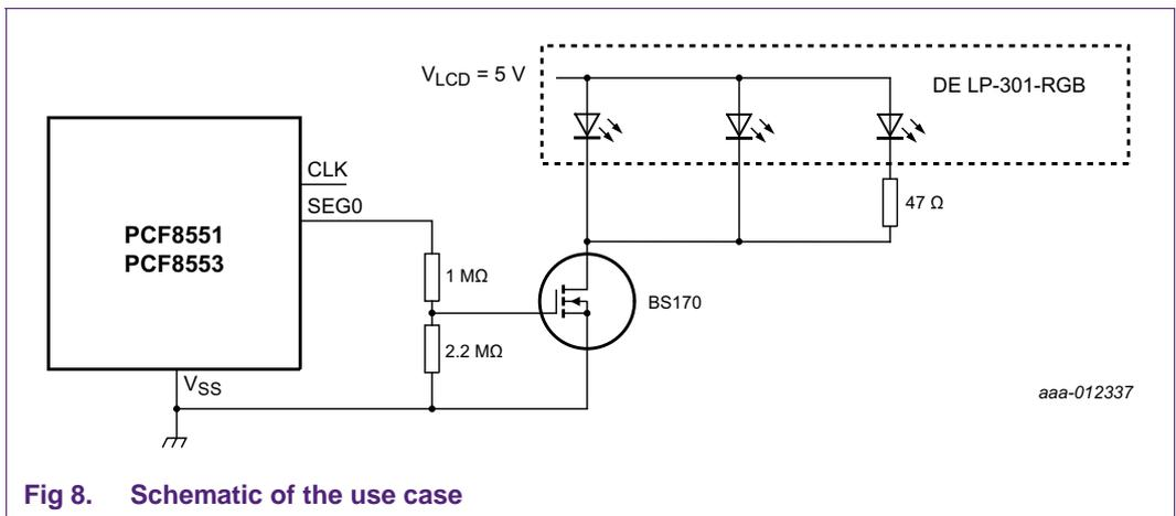
Fig 8. Schematic of the use case
