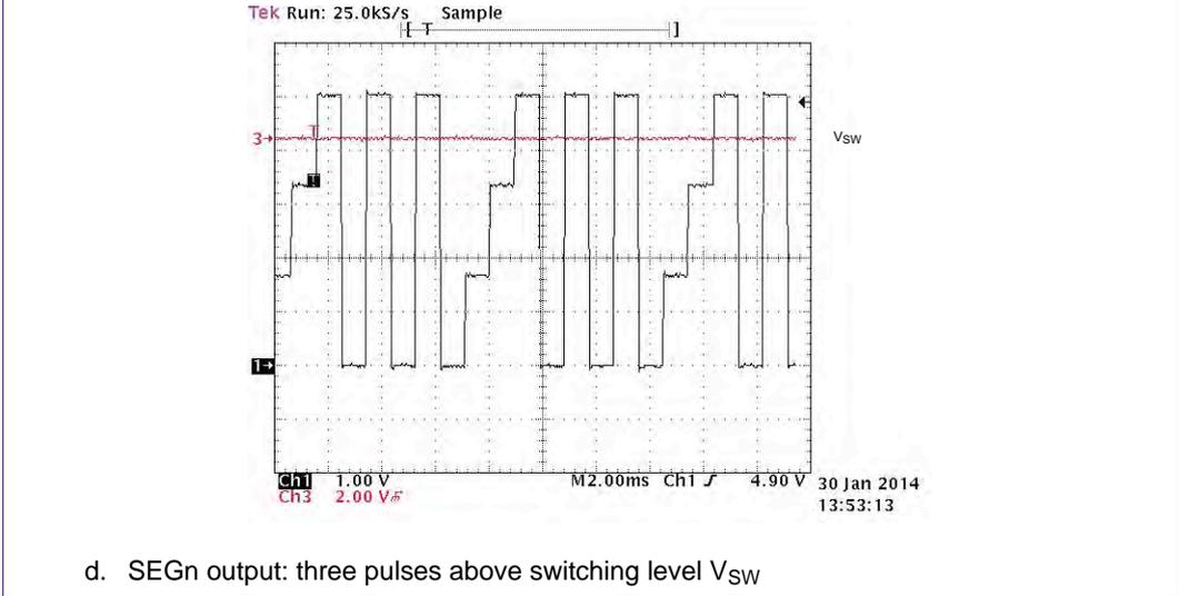
d. SEGN output: three pulses above switching level  $V_{sw}$
