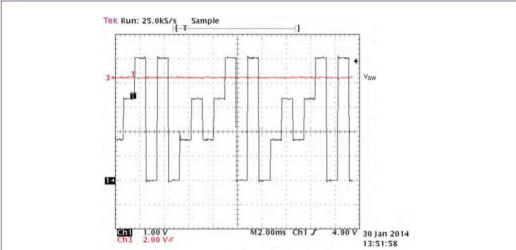
c. SEGN output: two pulses above switching level  $V_{sw}$
