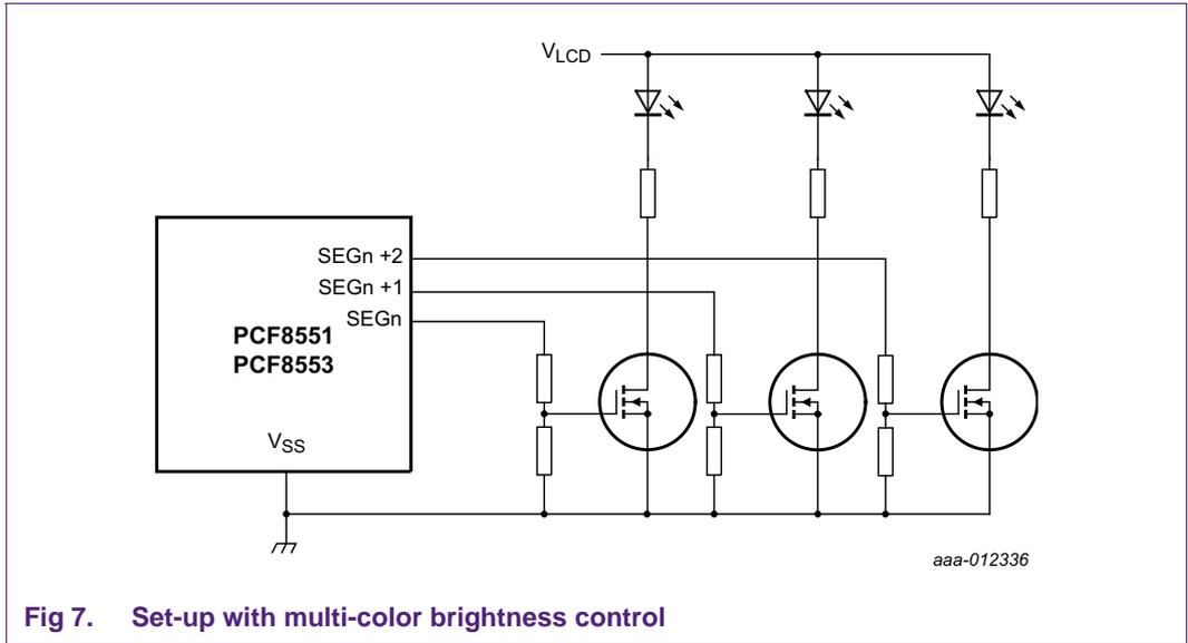
Fig 7. Set-up with multi-color brightness control
