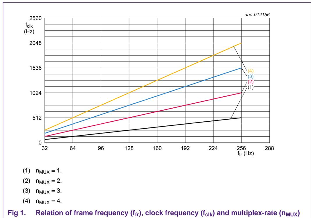
The clock frequency is set by writing to registers 01h and 02h. To feed the clock-frequency to the output, the COE bit must be set to logic 1.
