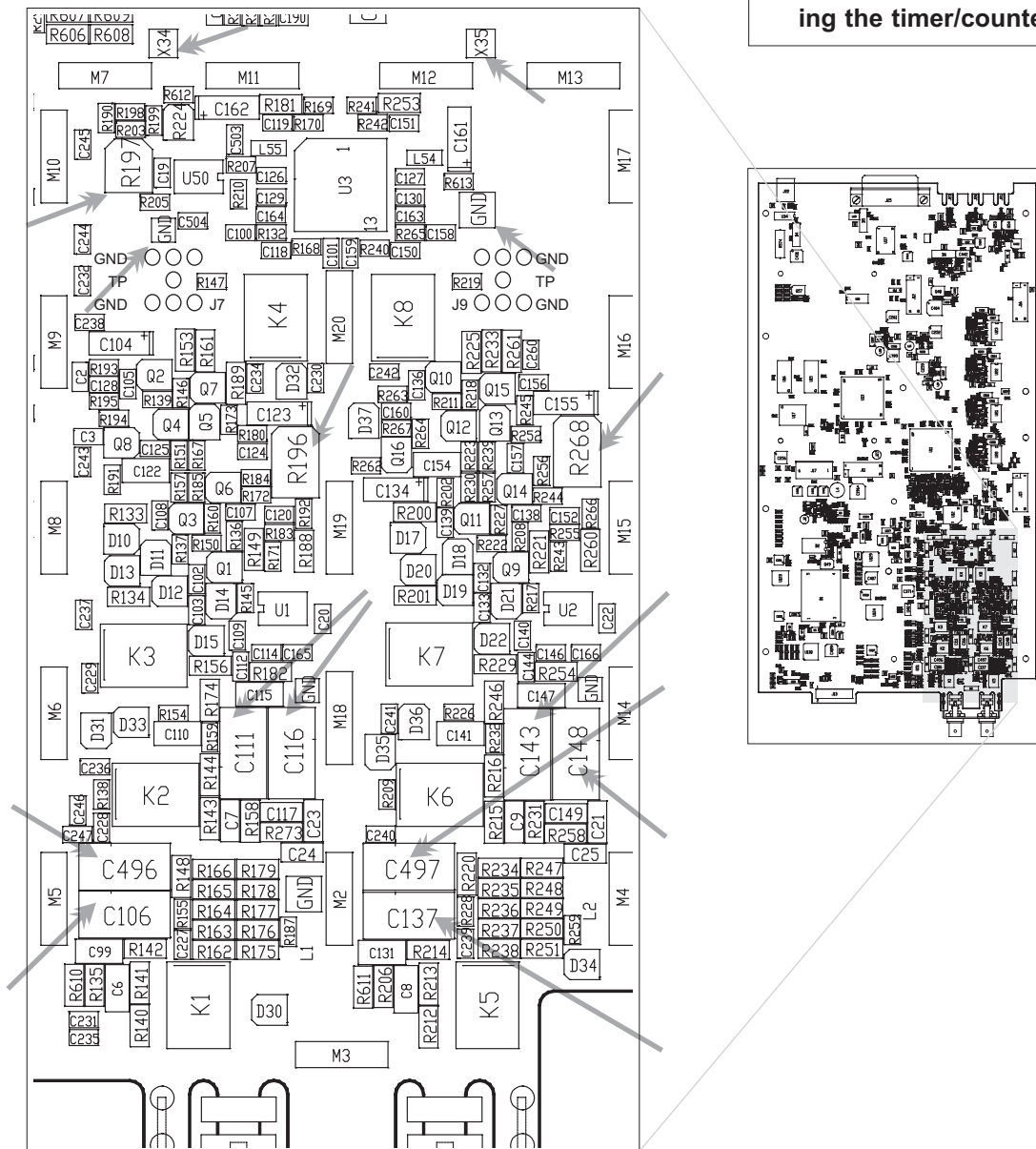
Figure 7-2 Test points and trimmers for the input amplifiers.
