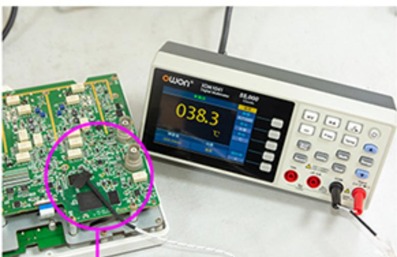
Built-in temperature sensor, auto cold junction compensation, display temperature in °C, °F or K, support K-type thermocouple.
