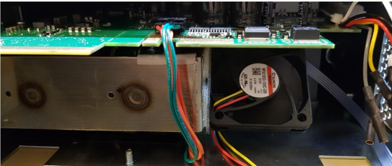
New mounting of original Fan at the end of the dual transformer pack using [3M Dual Lock](#).
