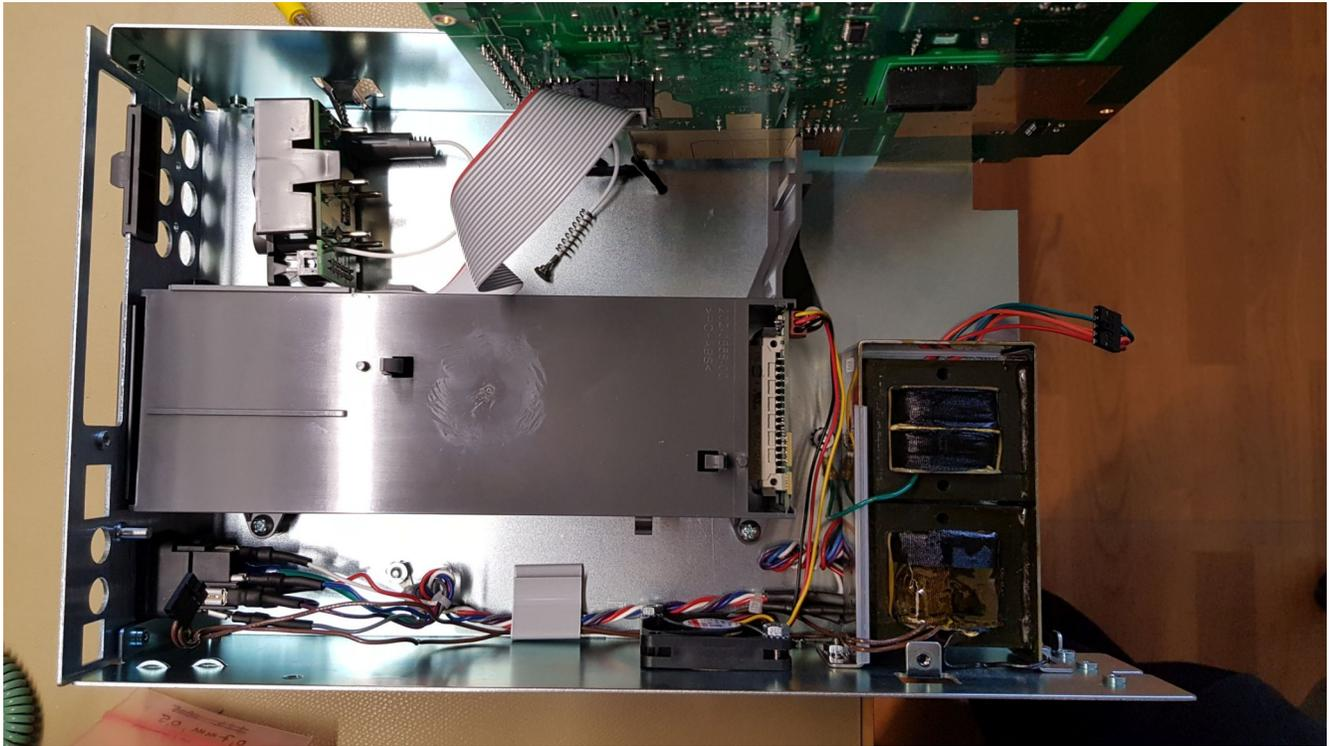
Main PCB removed. The big Gray box is the Expansion Slot with the two clips holding the Main PCB. Lower right, Dual Transformers One for the Digital Section and one for the Analogue section.
