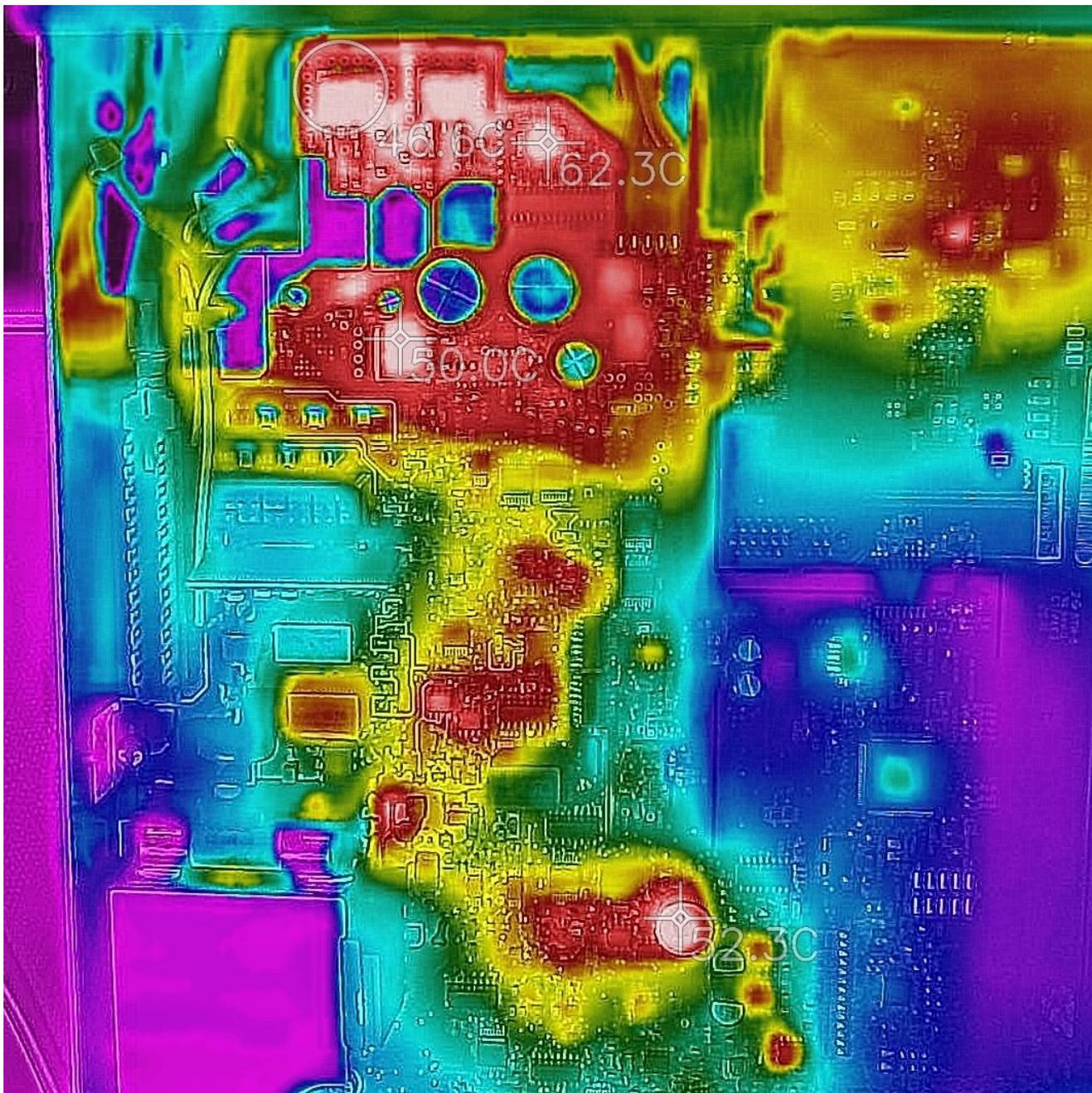
Open box, lid off and after 2 hours using a Flir One Pro. Highest temperature is 62C.
