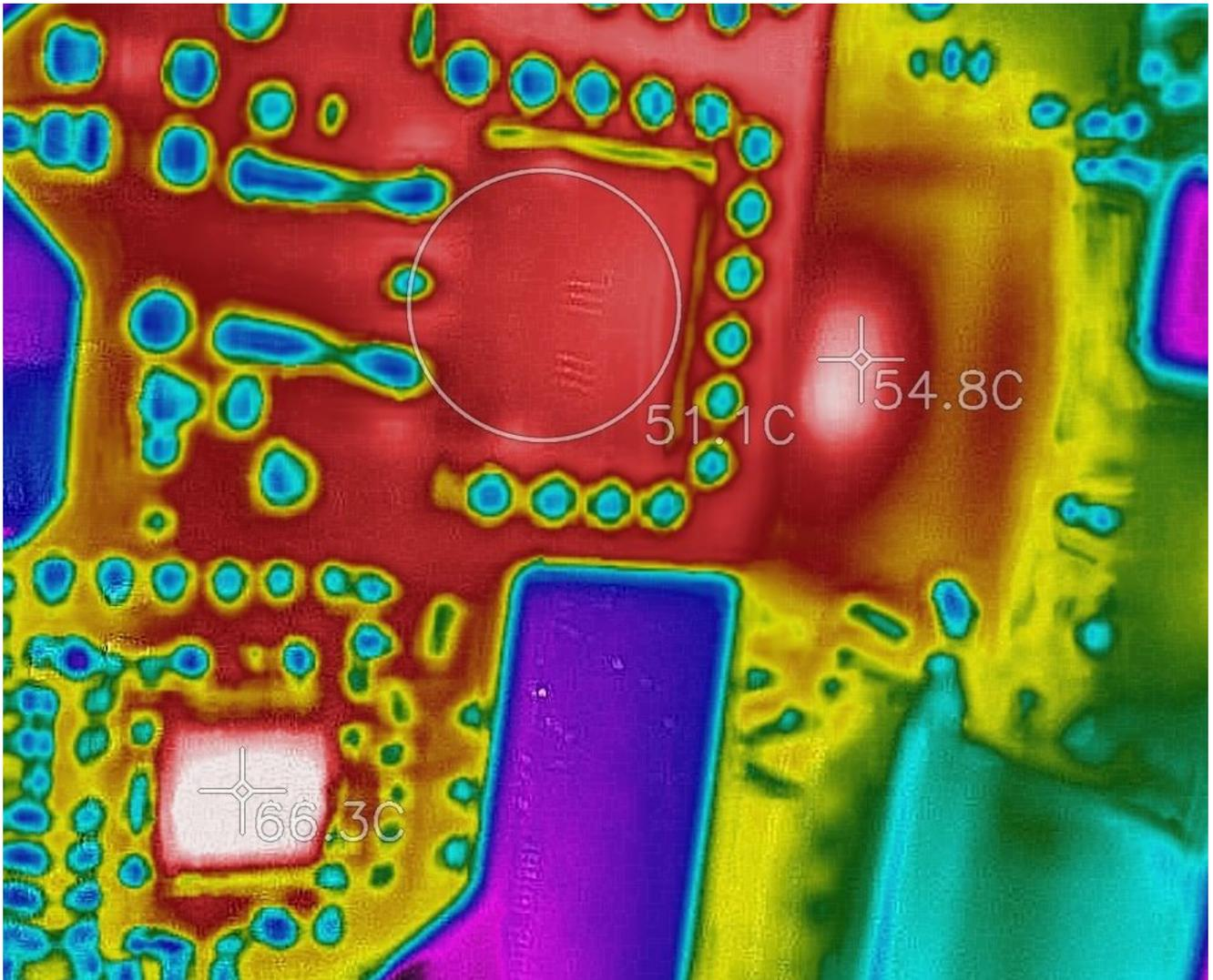
This is a bit hard to see but the left part is the Main PCB with the analogue voltage regulation section, 66.3C and 51.1C. To the right is the Front PCB with CPU etc. where one spot is reading 54.8C.
