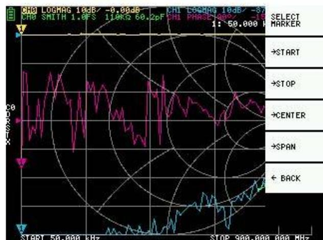
Up to 4 markers can be displayed. Markers are selected by the menu items **MARKER** → **SELECT MARKER** → **MARKER n**. Clicking on a disabled marker menu item enables it and makes it active. Clicking on an enabled but non-active marker activates it. Clicking on the currently active marker disables it.
