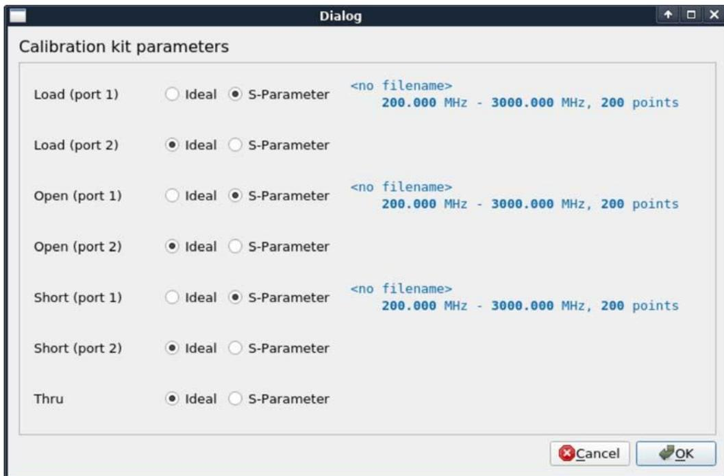
Each calibration kit type can be associated with an S parameter model, or an ideal model can be used. Clicking on the S-Parameter radio button will bring up a file chooser dialog to select the S parameter file.
