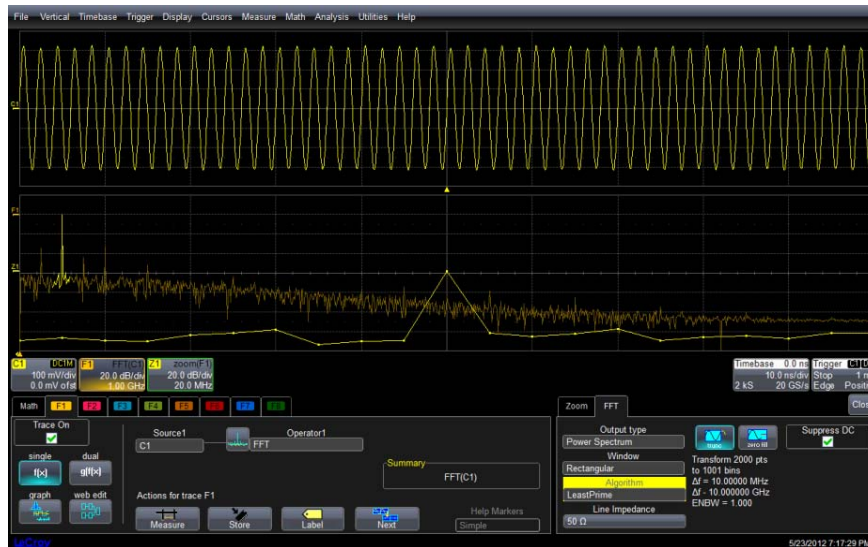
Figure 2: Frequency resolution @ 10ns/div
