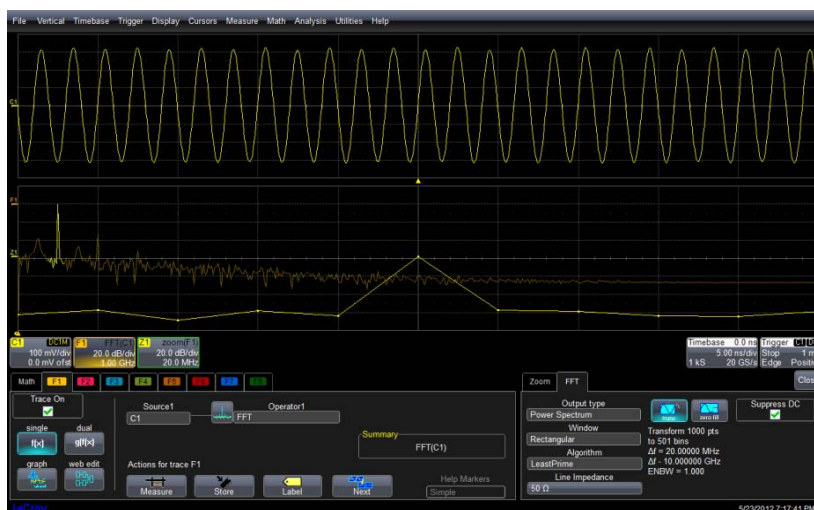
Figure 1 Frequency resolution @ 5ns/div
