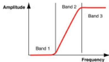
High-pass filters are useful for eliminating DC and low frequency components. Sample applications include Disk Drive and Optical Recording analysis (emulation of the SLICING function).
