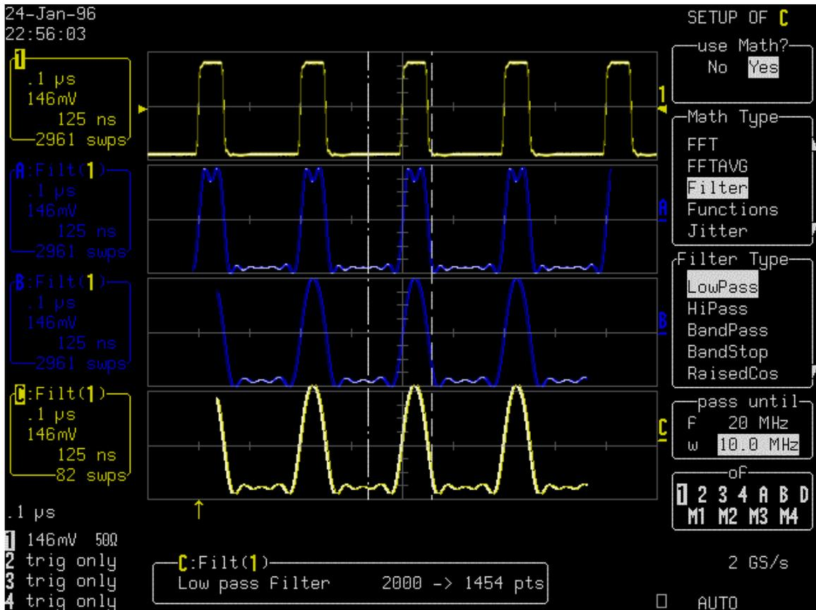
1: a signal composed of 5 MHz pulses is filtered by:
