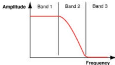
Low-pass filters are useful for eliminating accumulated high frequency noise and interference, and for canceling high frequency background noise.
