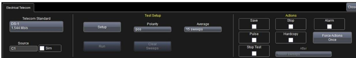
2. Touch **Telecom Standard** and select the desired standard. This will automatically set the requisite bit rate, mask, and pulse isolation criteria for the measurement.
