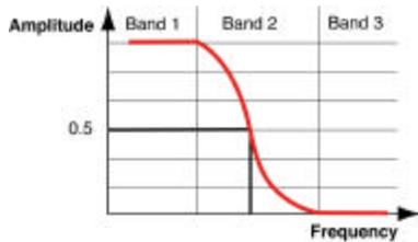
Band 1: Pass Band — DC to corner frequency minus half width; signal passes unattenuated.
