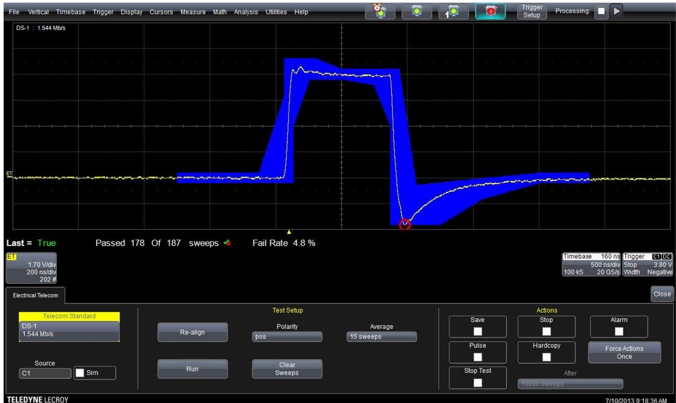
In cases where there are alignment criteria, such as a positive-going or negative-going pulse, the tests include settings to define these criteria, and the ET-PMT software will automatically find only those pulses.
