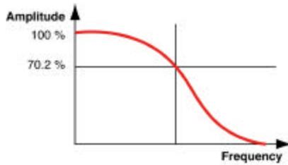
Band 1: Pass Band — DC to half power bandwidth% times modulation frequency, pass; 3 dB down at half power bandwidth.
