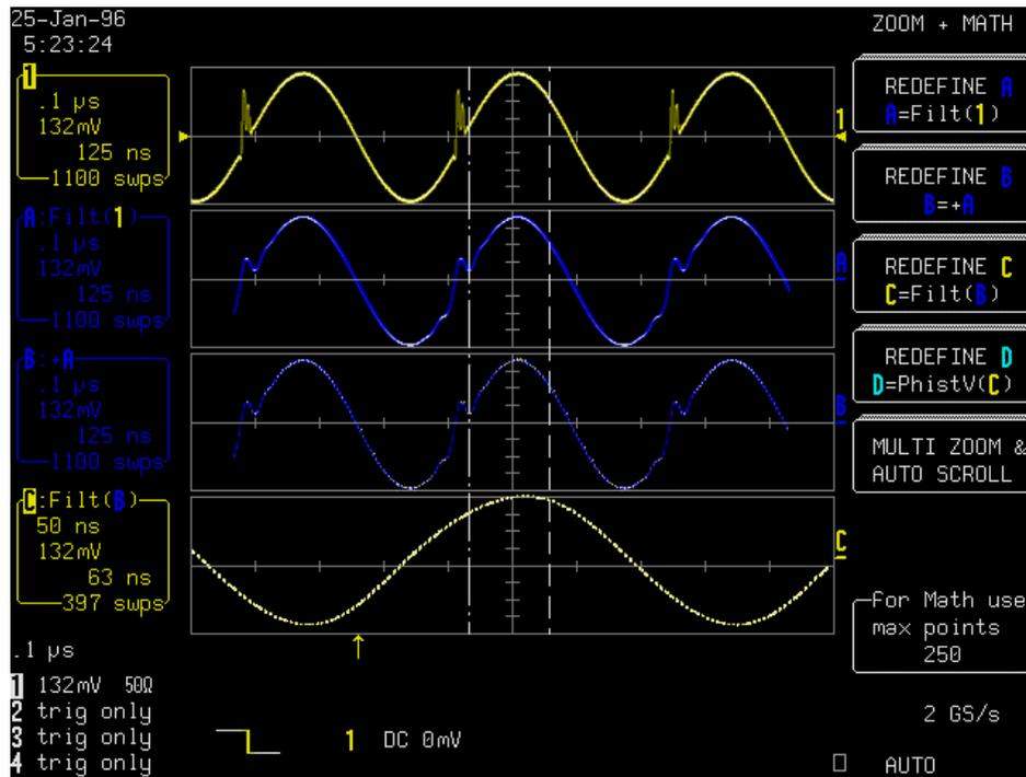
1. Channel 1 represents a noisy sine wave with a frequency of 3MHz.
