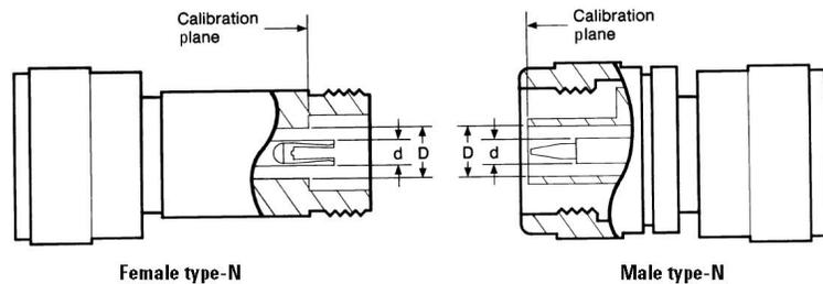
Figure 19. Type-N connector calibration plane
