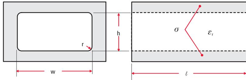
Figure 22. Rectangular waveguide dimensions and properties
