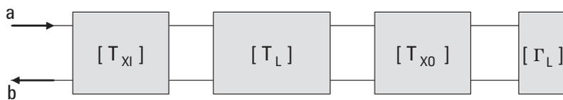
Figure 5. Cascade parameter representation of terminated transmission line model
