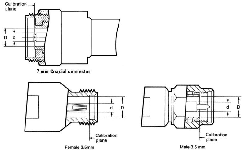
Figure 18. Location of coaxial connector calibration plane
