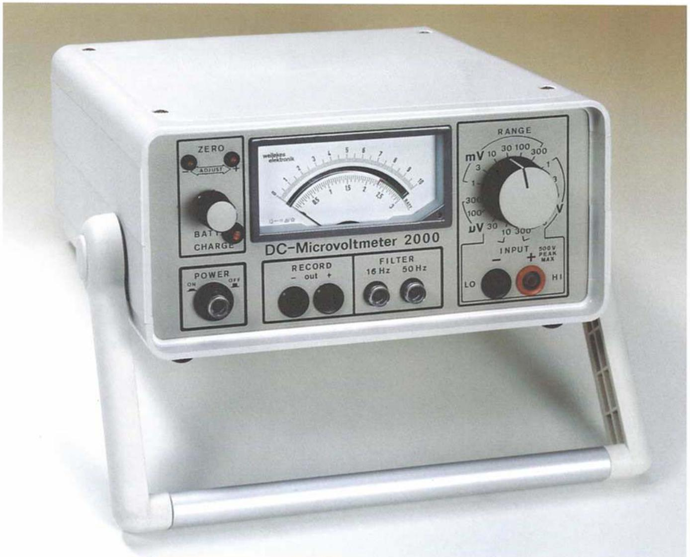
***Battery- and mains powered DC-Microvoltmeter
