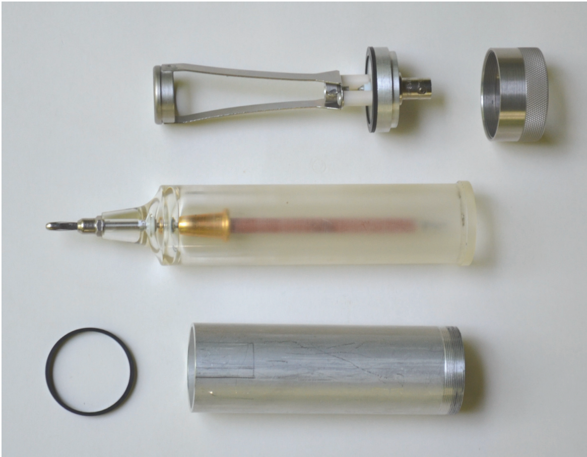
Figure 2. Disassembled probe tip.
