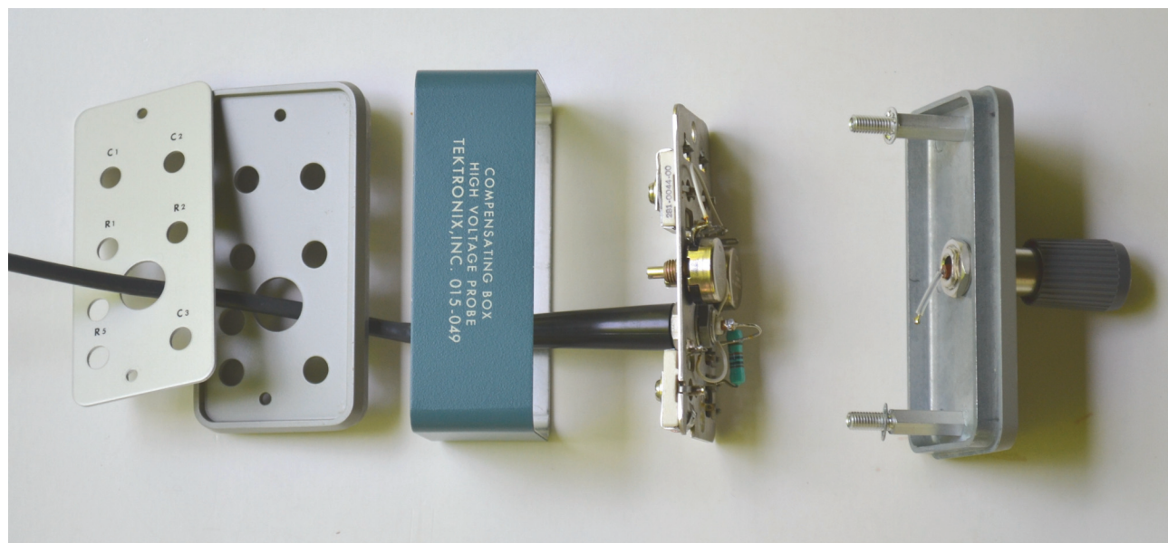
Figure 4. Disassembled compensation box.
