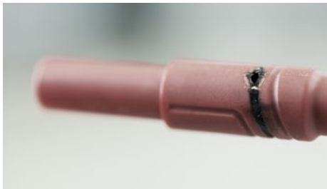
Breakdown with non-compliant plug-in connector
