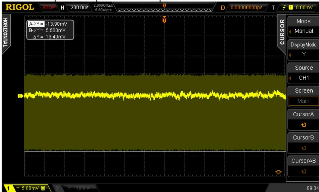
We see that the Earth's magnetic field may change the result by 20mV, or 200mA. So, CC-65 should not be moved during measurements.
