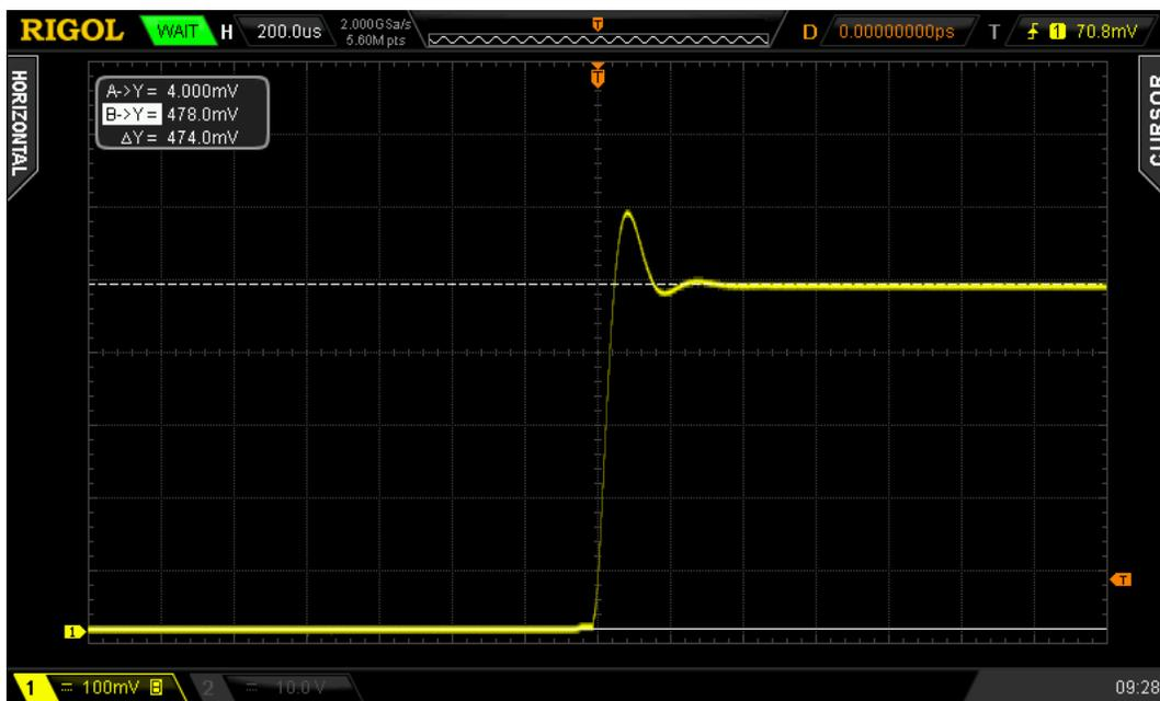
At the top of CC-65 current measurement range, 65A, current from the Source Meter is set to 5A.
