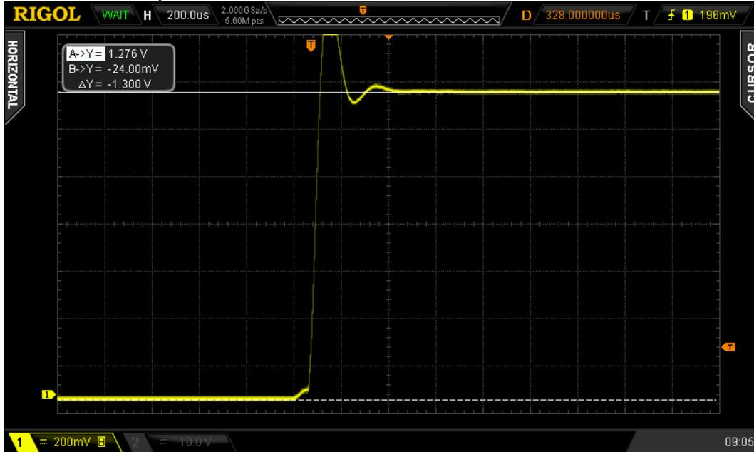
With 1.54A the measured current should be **20A**, and the voltage should be 1.77V. This, indeed, was observed. However, this seems to be **saturation level**. At 1.74A measured voltage should be 2.26V. In reality it takes large time, about 7 mS, for the voltage to reach 2.22V from fast step of about 1.8V:
