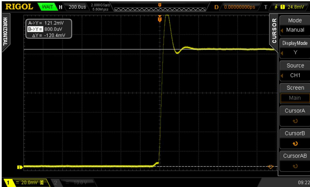
We see that at **1mV/100mA** the measured current is about 8% lower than the actual current
