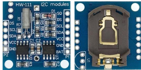
This second one is based on DS3231 and also has an AT24C32 EEPROM, but in this case pins 1-3 (A0-A2) are pulled up, so its default address is 0x57, which does not collide with the DSO's EEPROM. Also provides 3 solder jumpers (labelled A0, A1 and A2) in case you want to change the address by shorting them.
