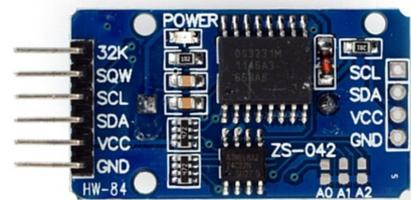
The DS3231 is more precise than the DS1307, as its internal oscillator is temperature compensated. For this compensation, it also includes a temperature sensor that can be read from the I2C bus, which would allow checking the internal temperature of the oscilloscope. This one can be found [for approx. \\$3,80](#) at the time of writing. Modifying the battery charging circuitry is also convenient in this module, as well as in the first one (see next section).
