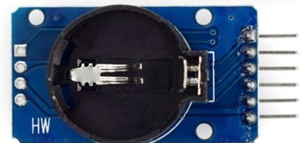
The third one [costs about \\$2,20](#) and is also based on DS3231, but this time it doesn't include an EEPROM. Its advantage is that it has the smallest footprint (barely bigger than the IC itself) and a rechargeable battery. It's so small that could be fitted on top the MCU so the internal temperature sensor could be used to check the MCU's temperature if overclocking, for example. This module doesn't need any modifications, as there's no EEPROM or external charging circuitry.
