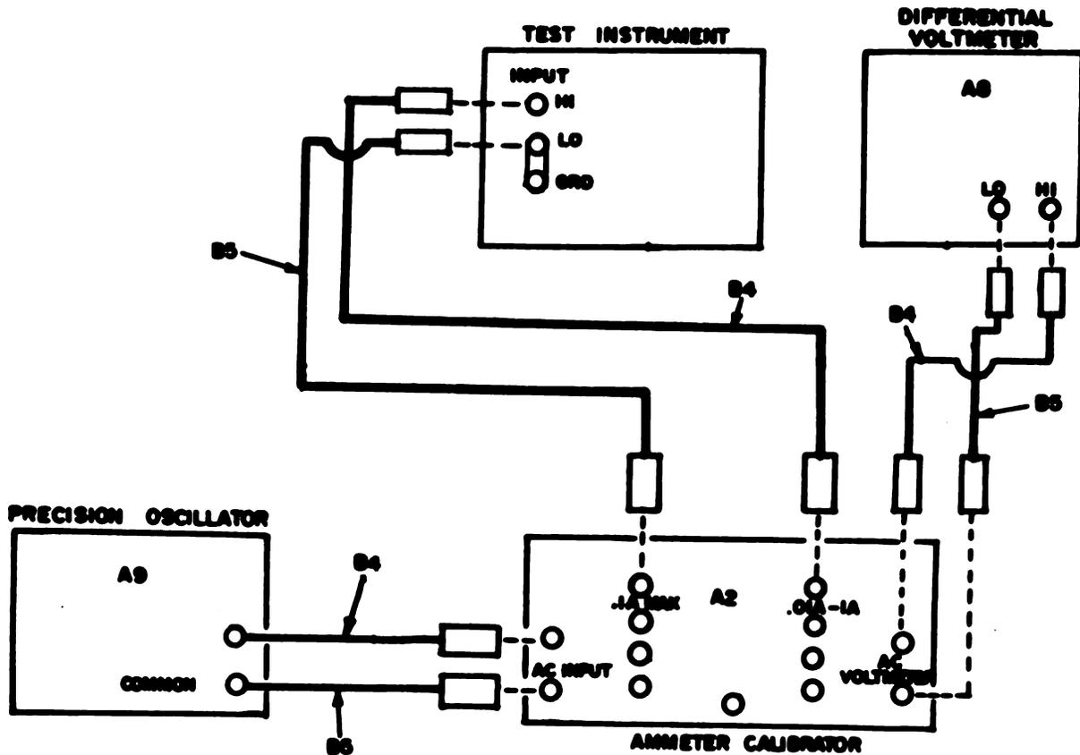
Figure 4. High ac current - equipment setup.
