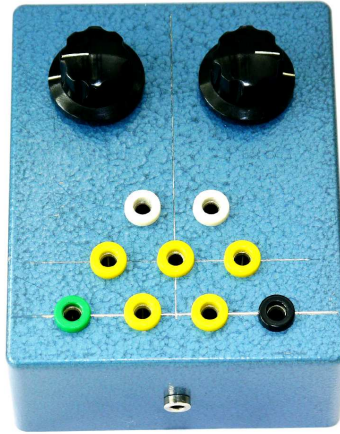
Figure 3.1. Picture of the top of the divider/switch-box. The instrument under test is connected to the two sockets closest to the switches. The voltage source is connected over the lower left and right sockets.
