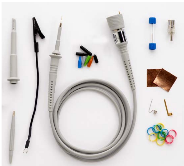
Figure 1. N2873A 500 MHz passive probe with standard accessories
