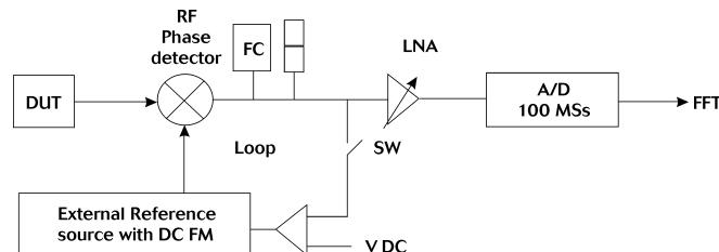
Using the built-in frequency counter, the LO reference source is tuned to the DUT frequency, while the switch 'SW' is in the open position. Then the beat signal between DUT and reference is used to calibrate the phase detector transfer function. Built-in automated functions measure the DUT frequency and tune the LO reference source to the same frequency.
