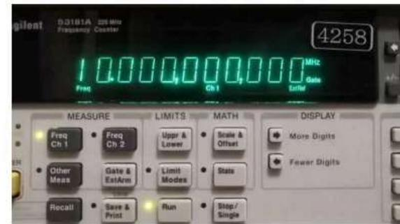
This photo is using an Agilent 53181A frequency meter and using a rubidium clock as the external clock and a 1S gate to test the GPSDO.
