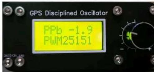
When used for the first time, it takes about 30 minutes to calibrate and correct. When the PPb value is observed to be  $0.0 \pm 1$ , press the encoding switch to enter the menu, rotate the encoder to find the "PWMSET" option and press the encoder switch to save the current PWM value.
