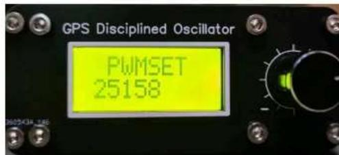
Rotate the encoder again, find "EXIT!! OK" and press the encoder switch to exit the menu. At this point, the calibration is basically completed.
