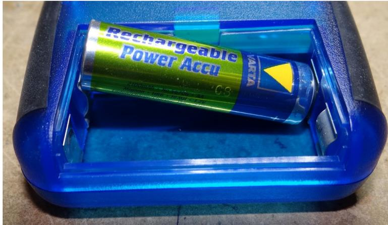
To get the cells back out, you can either put a piece of sticky tape around the negative end and leave a bit in the air before you install them and use it to pull them out, or bang the case on the heel of your hand to dislodge them.
