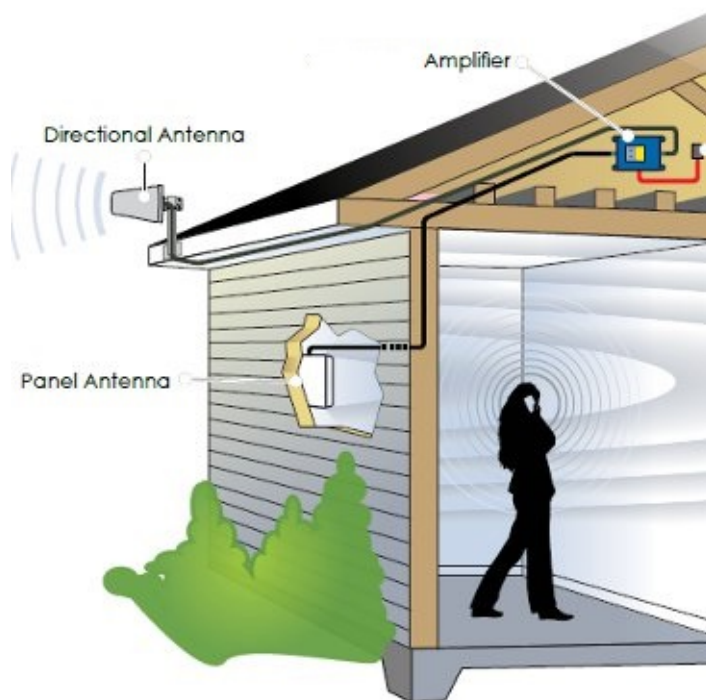
Figure 1: A typical bidirectional amplifier installation
