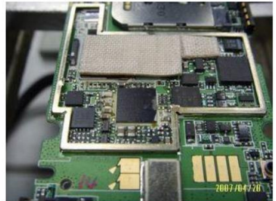
Stick the 6-layers prevent heat tape on PCB to prevent damaging Other ICs.
