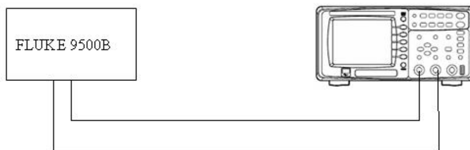
Picture 3-1 Connecting test instruments
