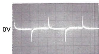
2 50 mV/cm, 5 \mu sec/cm PULSE PERIOD (PP) = 34.5 \mu sec SQW = 5.0V
