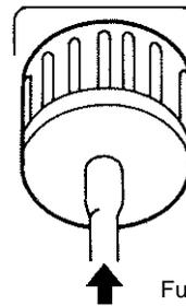
Fully insert the hose into the vacuum outlet cap.
