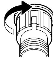
Secure the plug by turning it clockwise.
