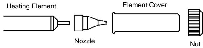
Remove the nut with the attached spanner.
