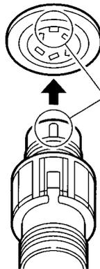
Insert the cord assembly by keying the plug to the key on the receptacle.
