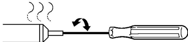
The cleaning pin passes cleanly and completely through the hole.
