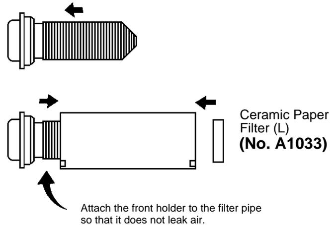
Firmly press the back holder assembly into the filter pipe in order to properly seat the O-ring against the pipe.
