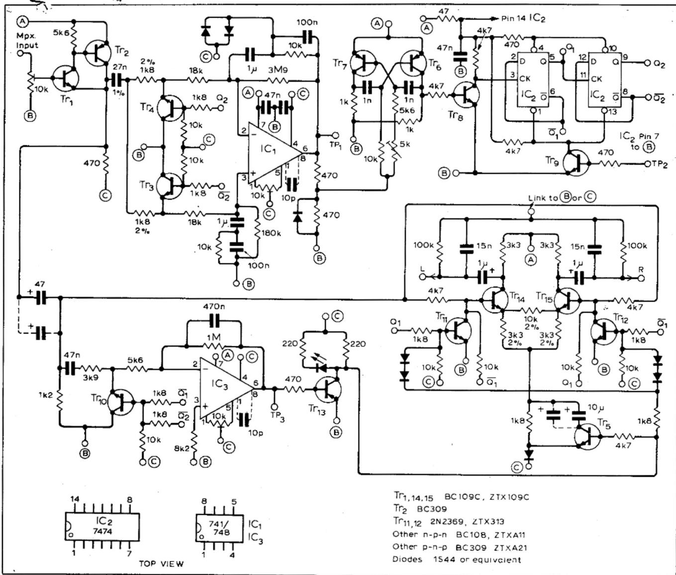
ough to avoid frequency jumping with various loads. This device is only intended for use on a fixed frequency and there is no varicap sensitivity or linearity correction. Calculation for this circuit suggests distortion at full deviation of less than 0.5%. For a fully tunable generator with calibrated attenuator the coder could be fed into the wideband modulation input of the Sound Technology FM1000 signal generator.
